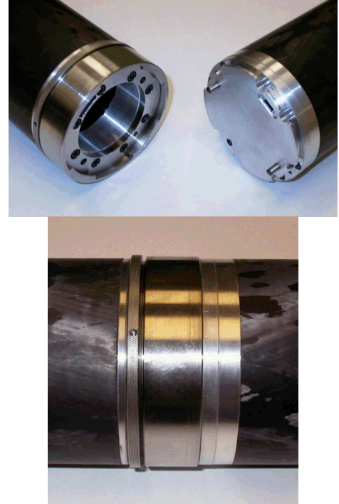
Figure 6: ARM Quick Connect Mechanism (open/closed)
