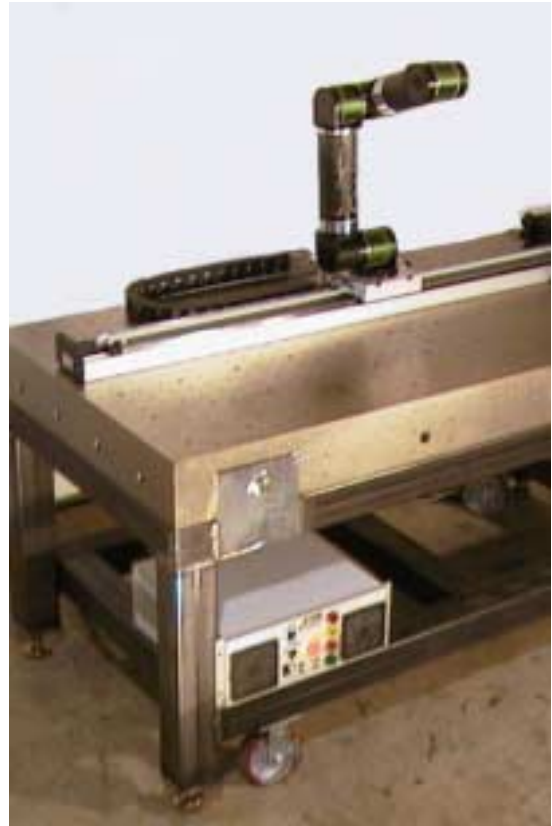
Figure 10: 3-DOF on Linear Track
