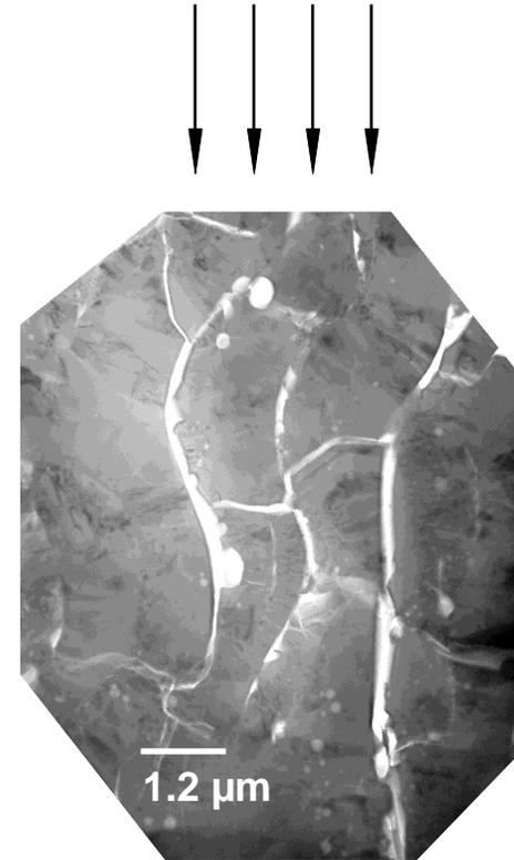
Sample fractured at 400 MPa
