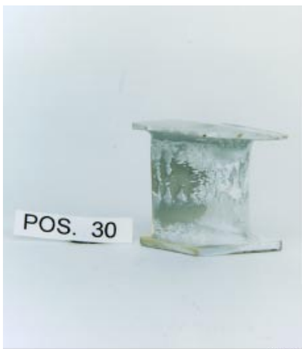
Figure 6. Ceramic material loss on convex surface.
