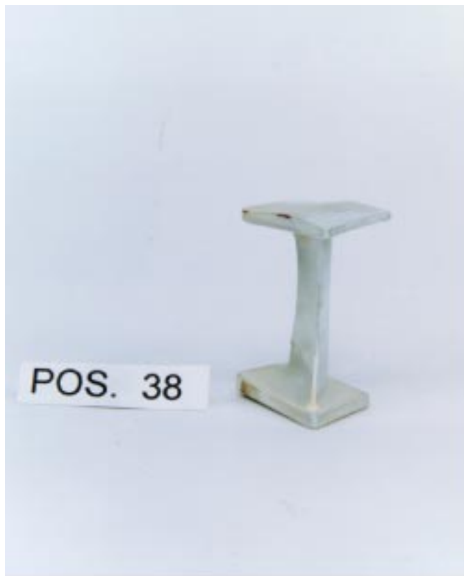
Figure 5. Ceramic material loss on concave surface.
