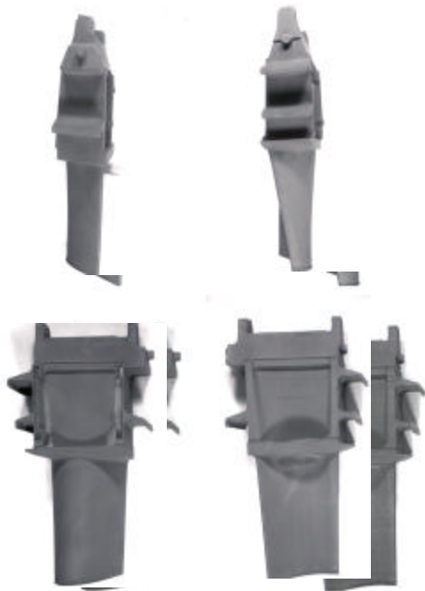
Figure 9 – Photos of defect-free 7FA Stage 1 Bucket casting.
