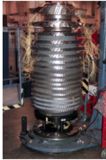
7H Compressor Rig Rotor (During Buildup)
