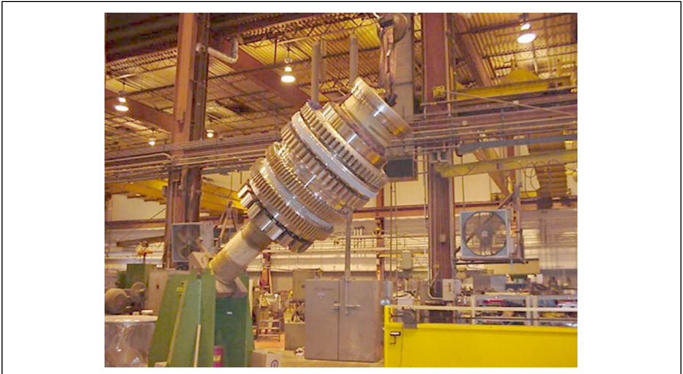
Figure 8. 7H Turbine Rotor During Assembly
