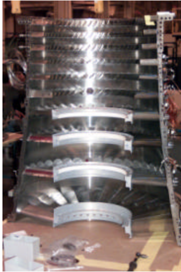
7H Compressor Rig Stator (During Buildup)
