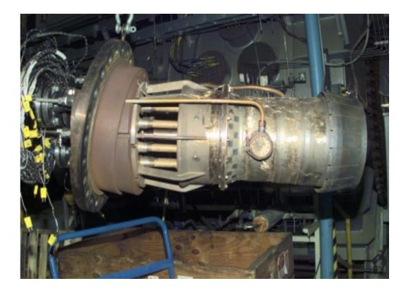
• Reactor integration into full combustor
