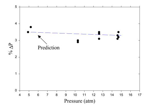
• 3.5% pressure drop at design conditions while fitting into existing envelope
