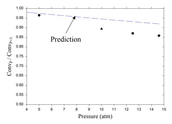
• 15 fold increase in pressure has small effect on reactor performance
