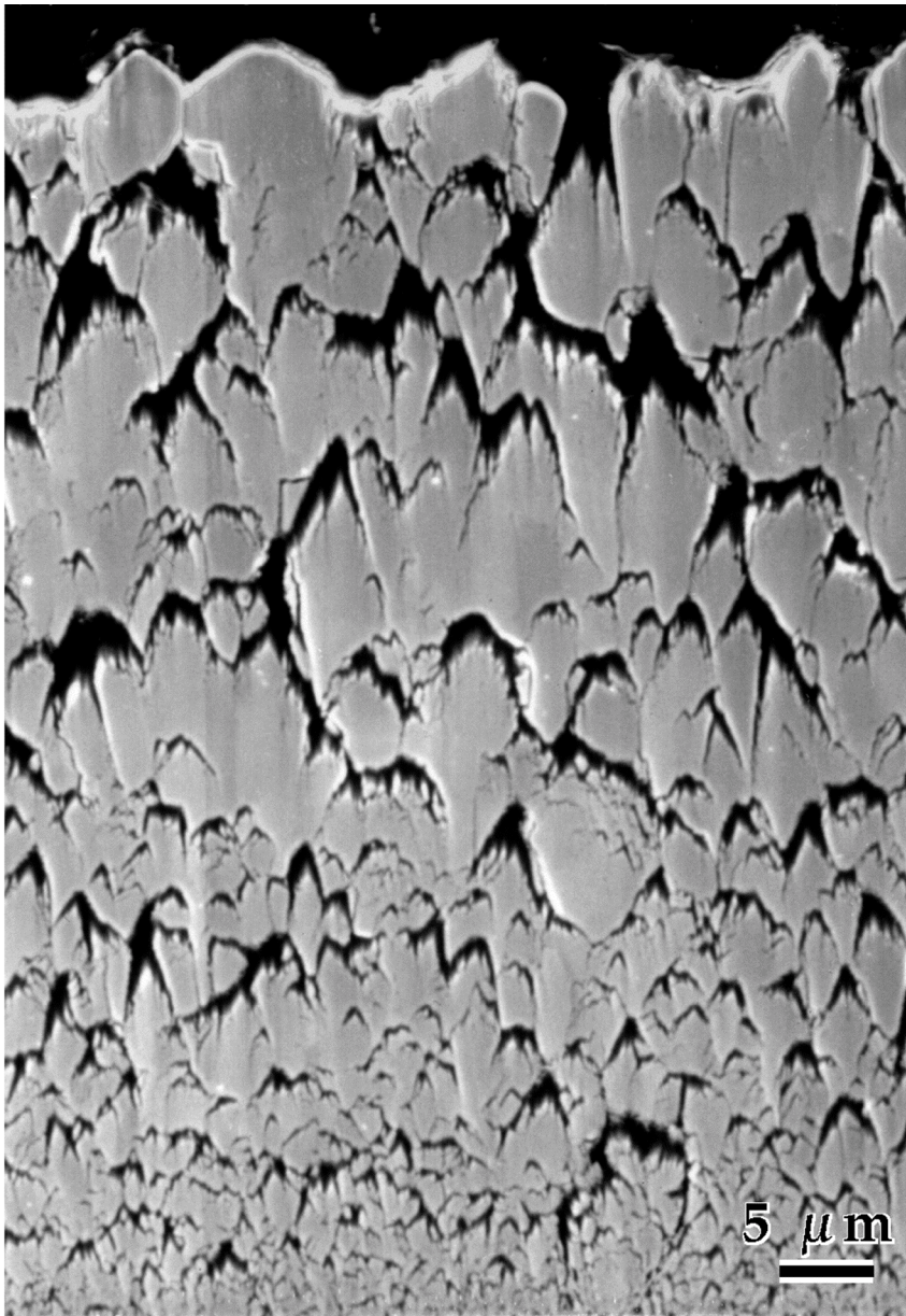
TBC Cross Section across Columns
