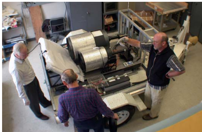
Goddard scientists installing the optics package for the KILT lidar. The larger telescope is the laser transmitter.
