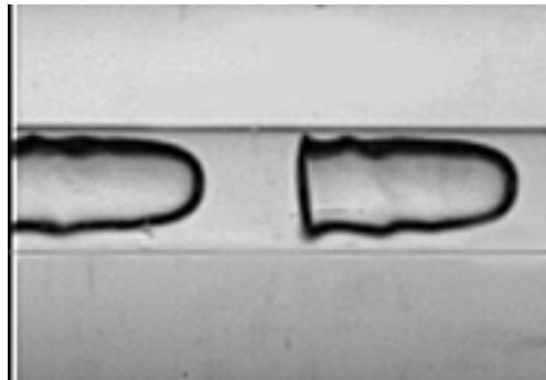
Fig. 2. Plug-slug flow in a 1 mm diameter tube flow. (Reprinted with permission from Int. J. Multiphase Flow .)
