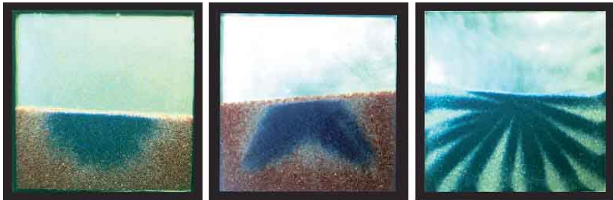
Fig. 6: Experimental results on quasi two-dimensional tumbling mixers with glass spheres of different sizes (0.8 mm blue, 1.2 mm clear, and 2.0 mm red). All three systems started well mixed and everything is equal except the degree of filling. From left to right: less than 1/2 full, 1/2 full, more than 1/2 full.
