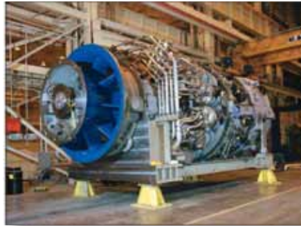
GE 7FB advanced technology gas turbine
