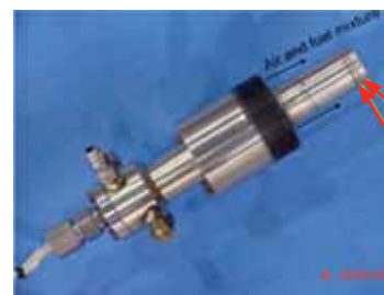
Top view with the mounting flange removed and the electrodes identified at the end of the exposed centerbody
