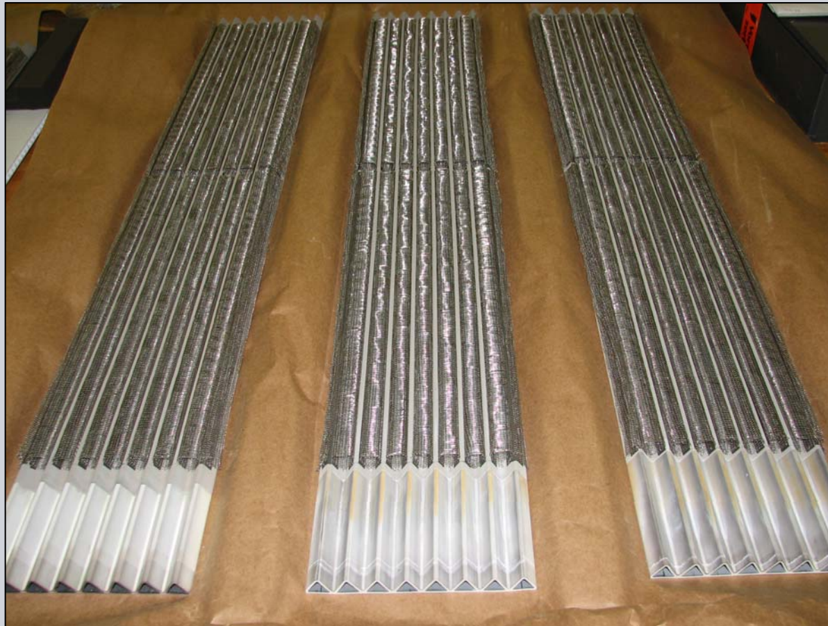
Delta8 cells with connectors in place
