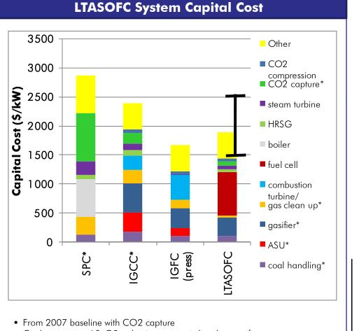
• Coal conversion / SnO2 reduction reactor is listed as gasifier
