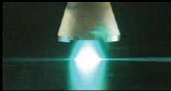
Droplet Measurements of a Diesel Reforming Injector Using Phase Doppler Particle Analyzer
