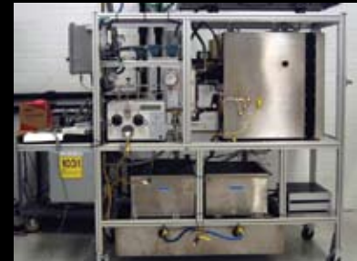
Test Rig for Analyzing Coke Formation of Fuel in Hot Environments
