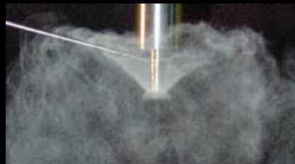
Piezoelectric Injector Developed for Low Flow Rate & Low Pressure Applications
