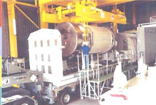
TN 52 DUAL PURPOSE CASK USED FOR ROUTINE TRANSPORTS
