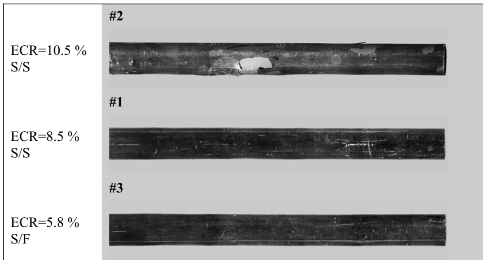
Fig. I-2. Appearance of E110 commercial irradiated claddings after a double-sided oxidation at 1100 C and S/S, S/F combinations of heating and cooling rates
