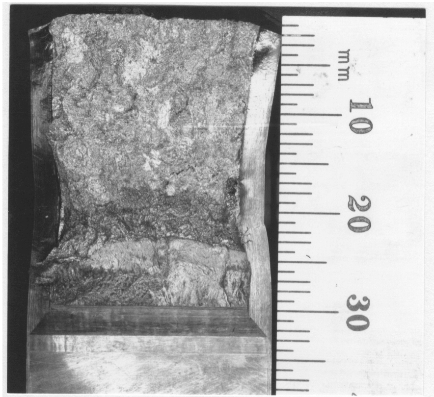
Figure C-32. Fracture surface of recovery-annealed material from the pump volute PV tested at room temperature
