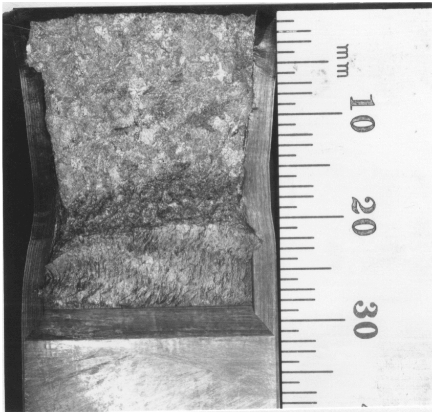
Figure C-14. Fracture surface of the hot-leg main shutoff valve MA1 tested at room temperature after 13 y of service at 281°C
