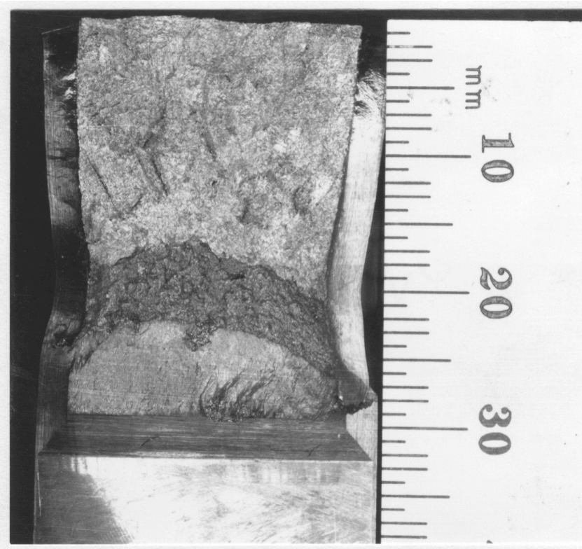
Figure C-44. Fracture surface of pump volute PV tested at 290°C after 13 y of service at 264°C
