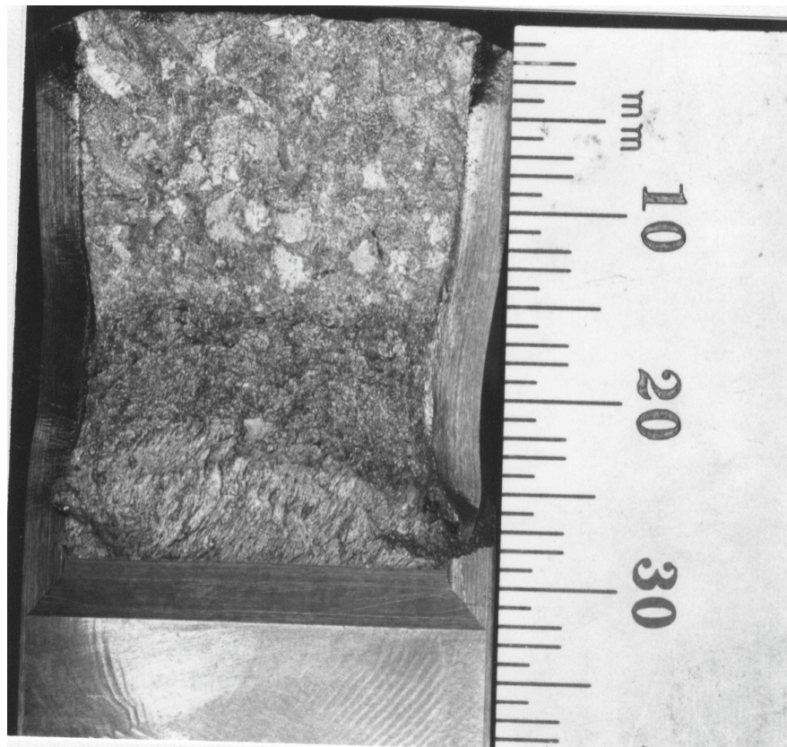
Figure C-23. Fracture surface of MA9 material from cooler region of the hot-leg main shutoff valve aged 10,000 h at 400°C and tested at 25°C
