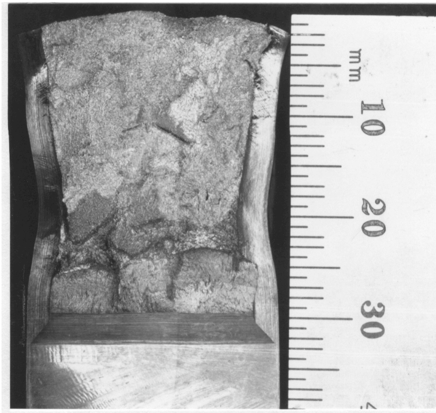
Figure C-35. Fracture surface of pump volute PV tested at room temperature after 13 y of service at 264°C
