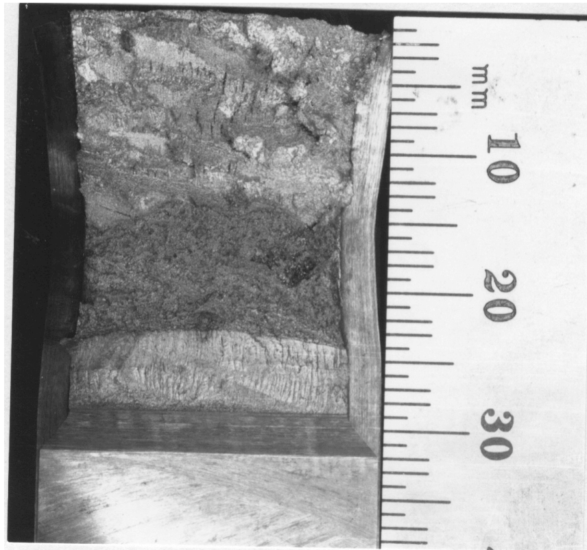
Figure C-8. Fracture surface of recovery-annealed material from the cold-leg check valve CA4 tested at 290°C
