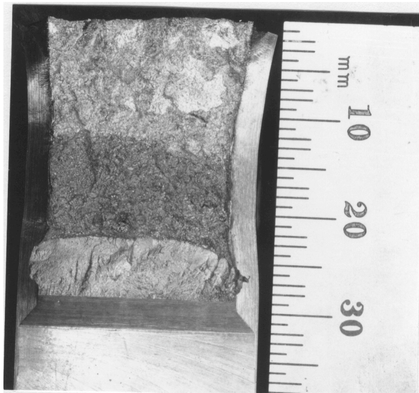
Figure C-56. Fracture surface of the unaged spare pump volute VR tested at 290°C
