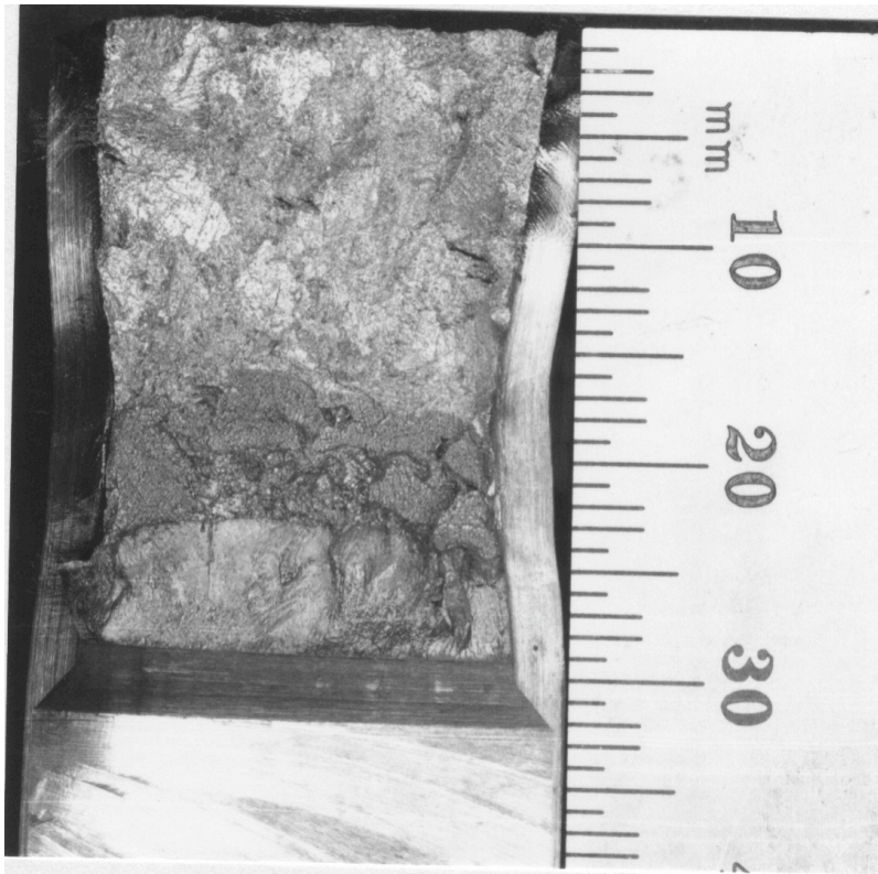
Figure C-41. Fracture surface of recovery-annealed material from the pump volute PV tested at 290°C
