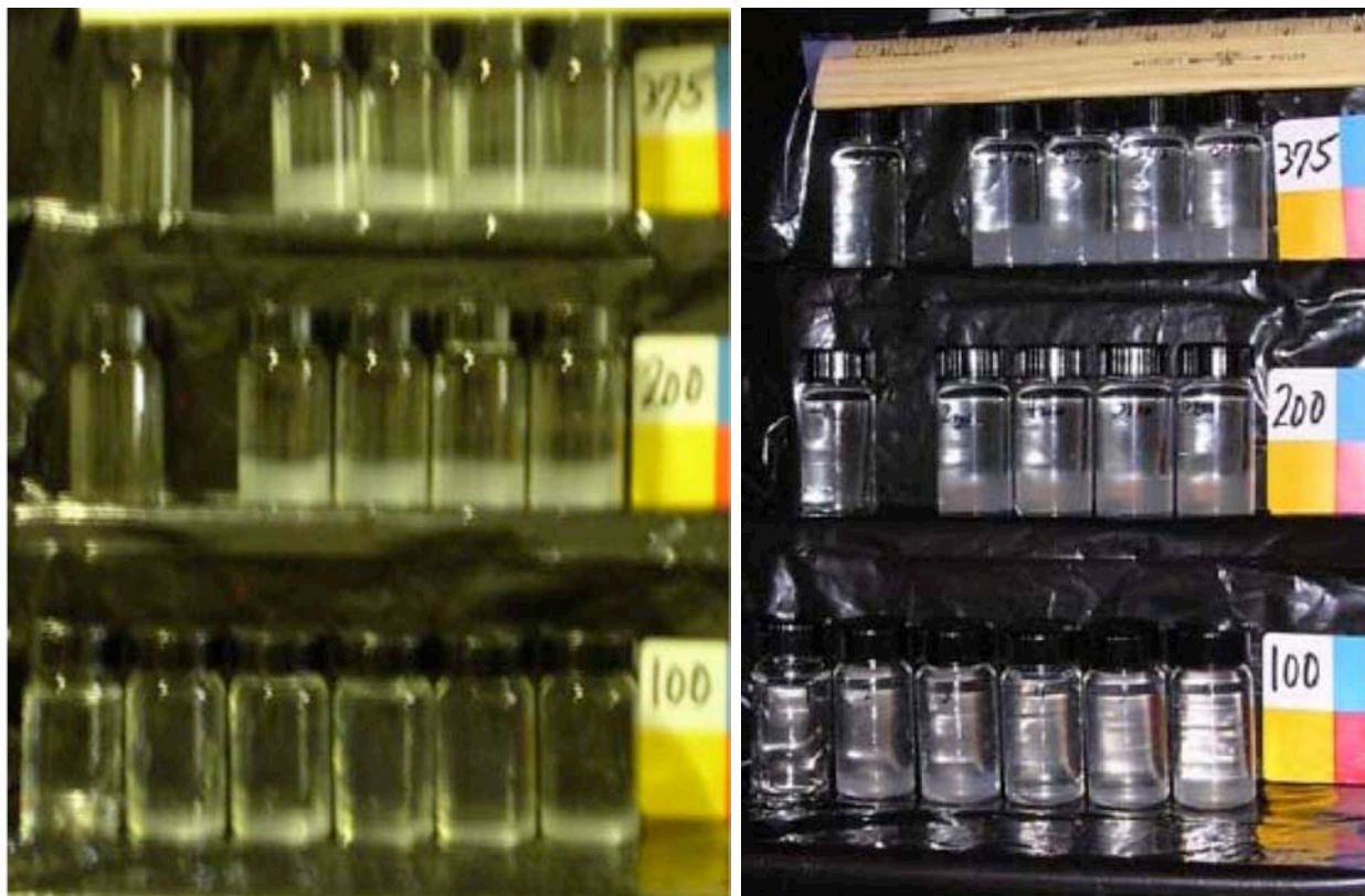
Figure 52. \text{Al}(\text{NO}_3)_3 100, 200, & 375 ppm surrogates. The photo on left was taken without flash to heighten the contrast between sediment and supernate. The photo on the right characterizes better the semi-translucent nature of the sediment. The bottles on the far left in each photo have no Al additions.
