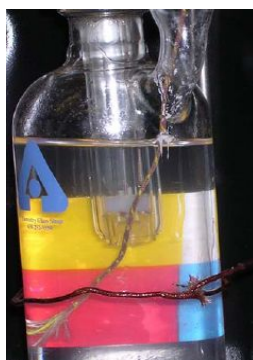
Figure C7. NaAlO 2 solution at T = 22.9°C, time = 450-min
