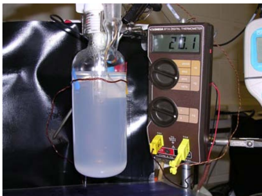
Figure C17. 17-h later at RT, a rather clear, transparent emulsion cloud occupies about 15% of the volume at the bottom of the flask.
