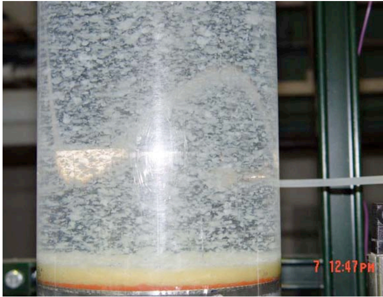
Figure 57. “Snowfall” as \text{Al}(\text{NO}_3)_3 solution was added to the loop.
