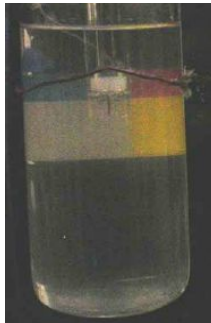
Figure C11. \text{NaAlO}_2 solution at 38.9^{\circ}\text{C} , still clear. Cooling time = 90-min.
