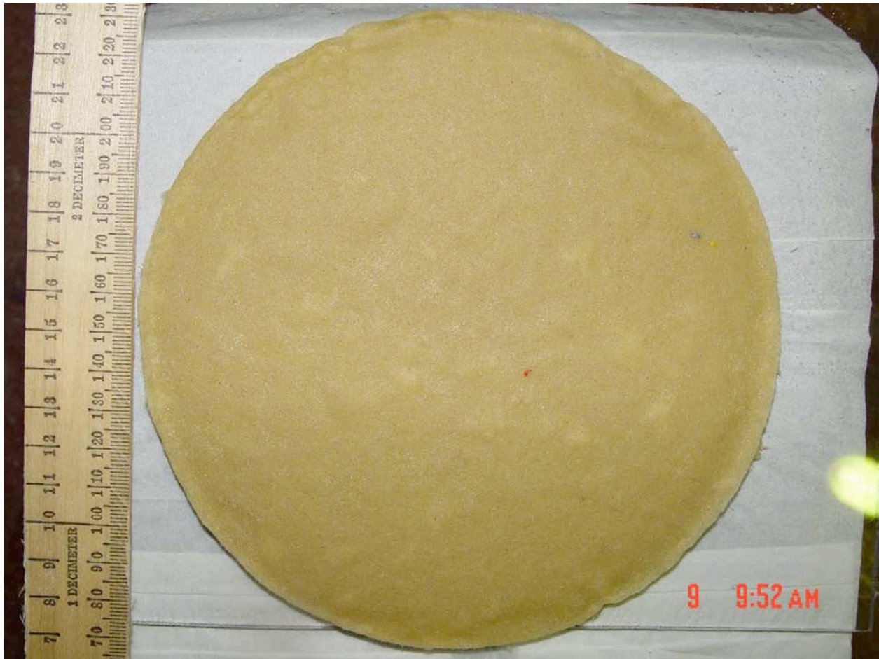
Figure 26. ICET-3-12 bed after removal from the loop. The smooth appearance is typical of the beds in the tests.
