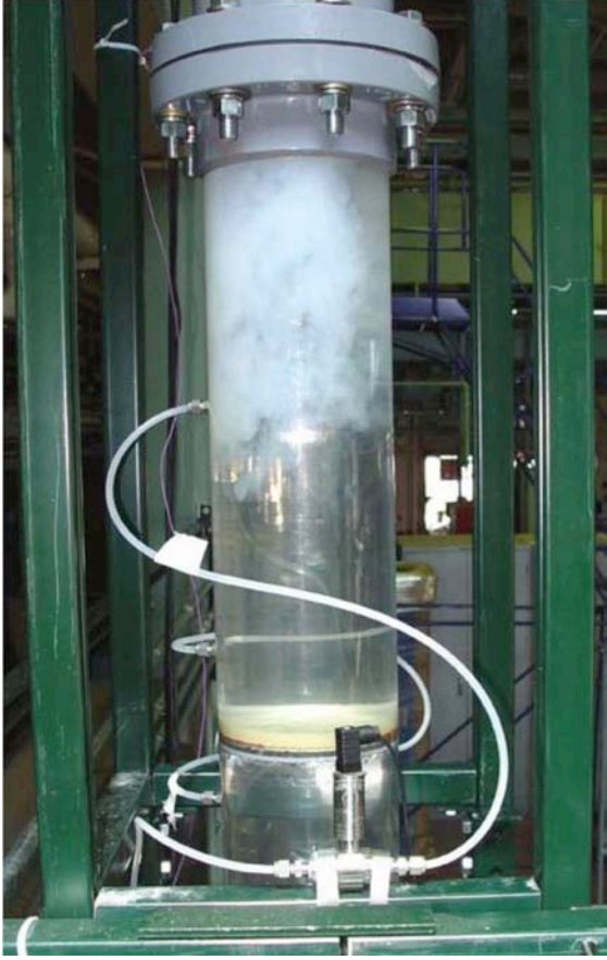
Figure 5. \text{Ca}_3(\text{PO}_4)_2 forming after addition of \text{CaCl}_2 and approaching the debris bed.
