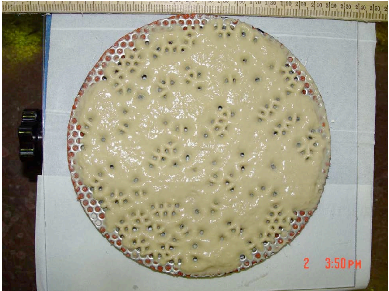
Figure 33. Plan view of debris bed formed by pure Cal-Sil loading in ICET-3-19-A2.
