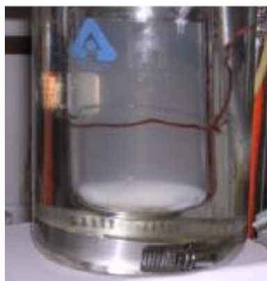
375-ppm-Al by adding NaAlO 2 Solution cloudy and undissolved sediment at the bottom
