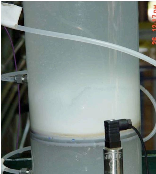
Figure 6. Precipitate buildup on the fiber debris bed just after the pump was turned off.
