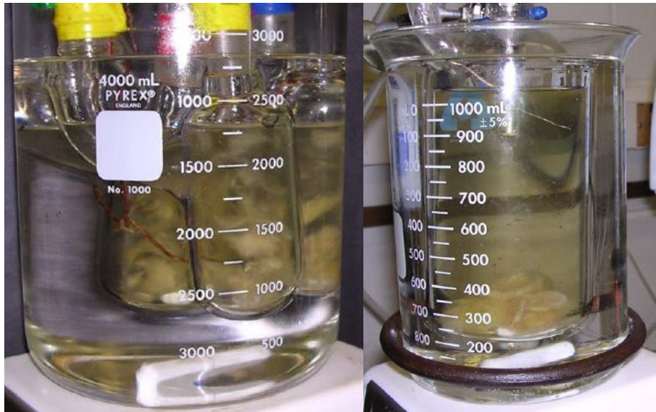
Figure E4. On the left are the tests in NaOH, TSP, and STB solutions at 48-h. The NUKON floats due to the bubbles becomes stick on the fiber surface. On the right side is the Al/NaOH test. The NUKON remained at the bottom of the chamber through the whole test period.
