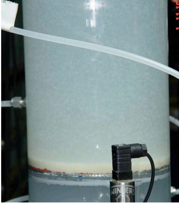
Figure 8. Flocculent precipitates observed at 0.01 ft/s in ICET-3-2
