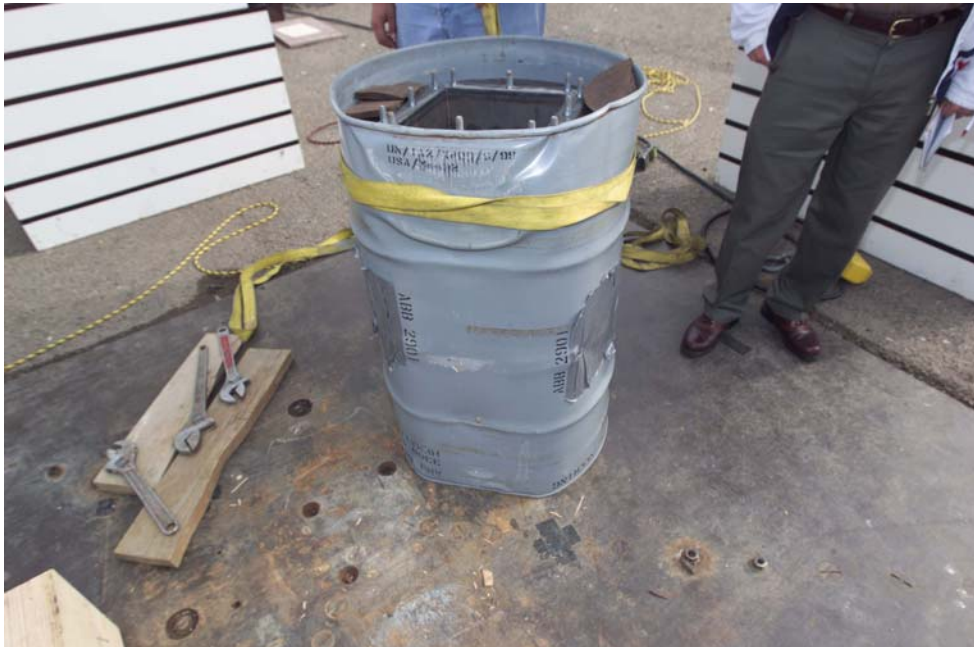
Figure 38. Damage to Open Drum, Side View
