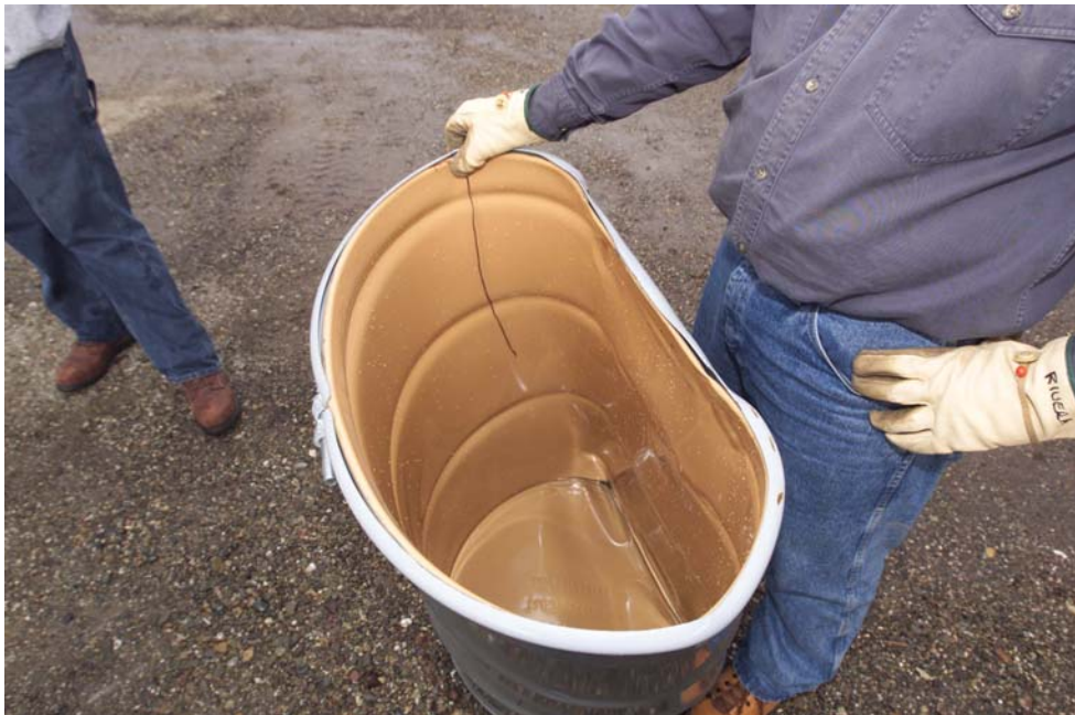
Figure 22. Damage to Drum (Ice-Filled Drop) Rich Villafana (LLNL) and Jesse Rivera (LLNL)
