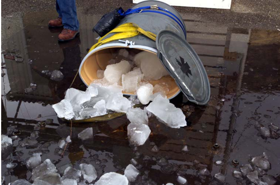
Figure 21. Damage to Drum and Lid after Ice-Filled Drop (Close-Up)
