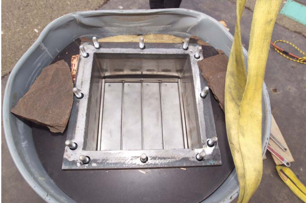
Figure 32. Inner Compartment, Upper Block Removed
