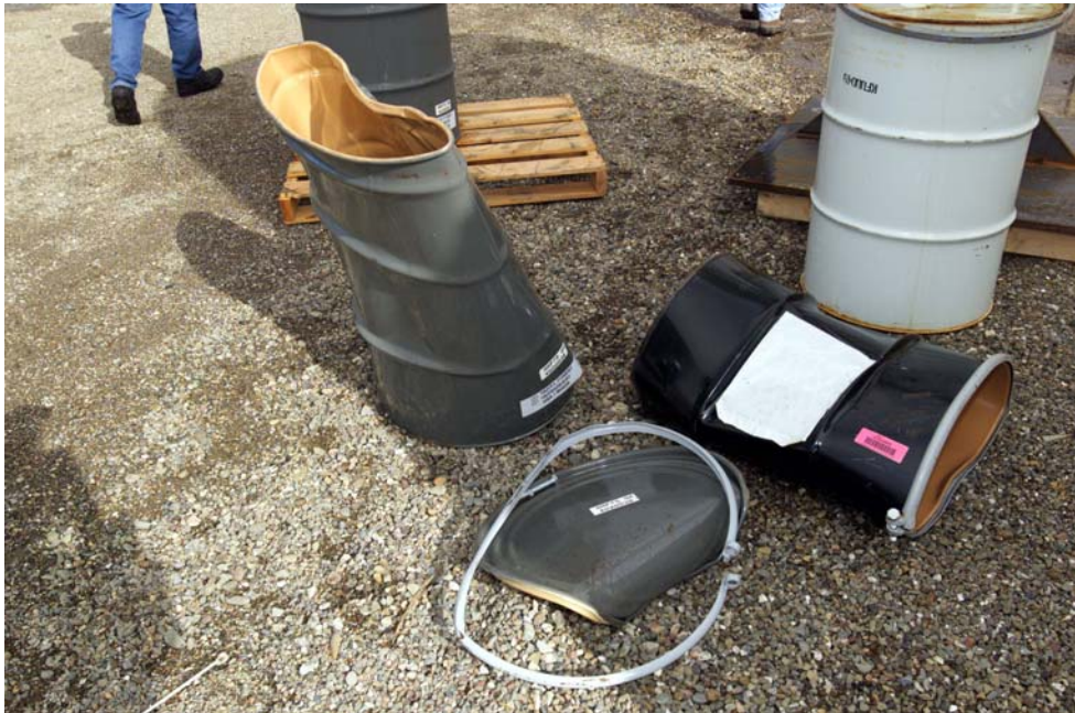
Figure 20. Damage to Lid, Closure Ring and Drum Along Side of Damage to Previously Dropped 133-l (35-gal), Water-Filled Drum
