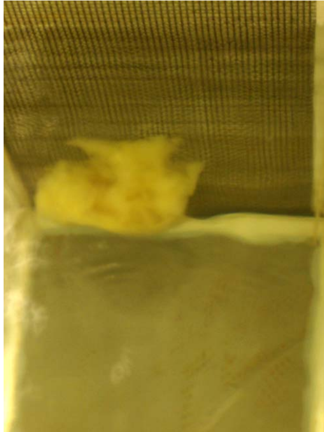
Figure 5-4. LS NUKON™ forms clusters at the test screen.
