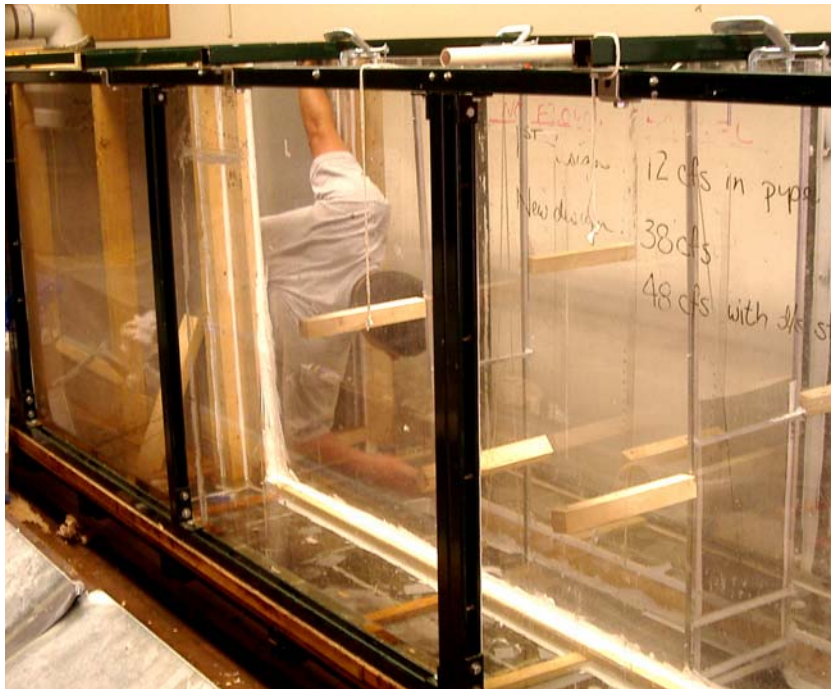
Figure 4-2. Removal of RMI by hand inside the flume.
