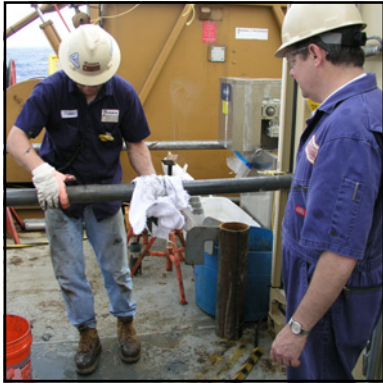
Example of the transfer of a hydraulic piston core into the core processing van
