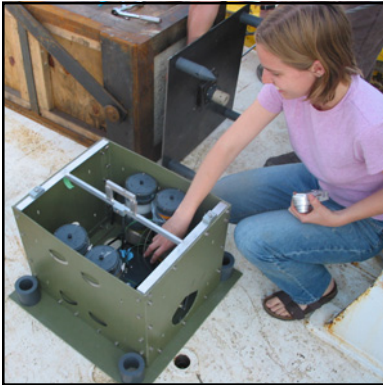
Laura Lapham (University of North Carolina) making the final predeployment check of the osmopumps, key components of the PFA
