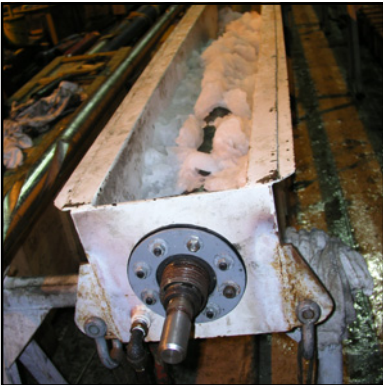
A pressure core on ice awaiting transfer to the van.
