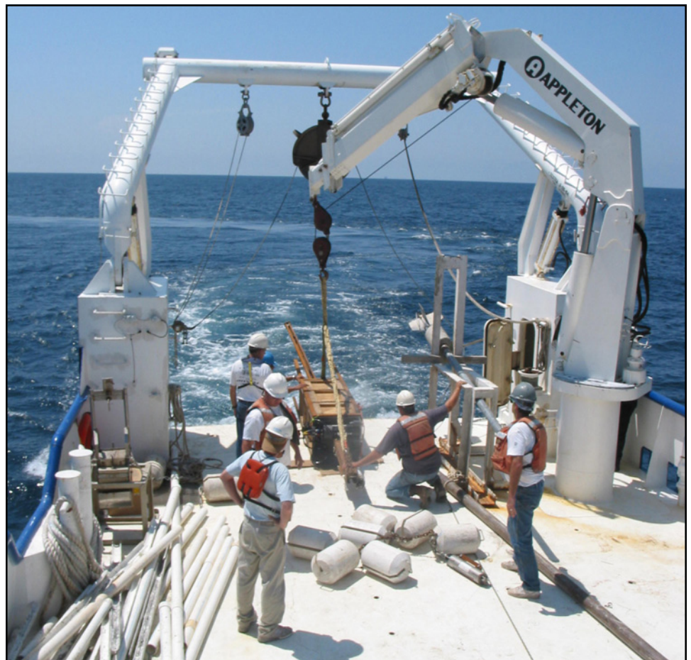
Deployment of the Pore-Fluid Array (PFA)
