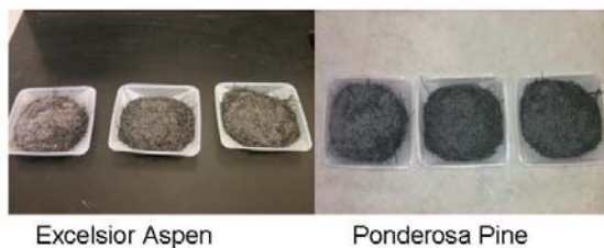
Figure 8. Ash from Aspen excelsior and Ponderosa pine needles that were treated with fire retardant chemicals prior to standardized combustion tests. Fish were exposed to a 1 percent solution of ash for 96 hours.
