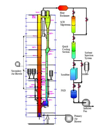
Schematic of circulating fluidized-bed combustion (CFBC) systems.
