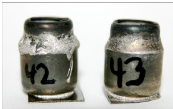
Figure 1. Successful Braze of Membrane Alloy to Stainless Steel
