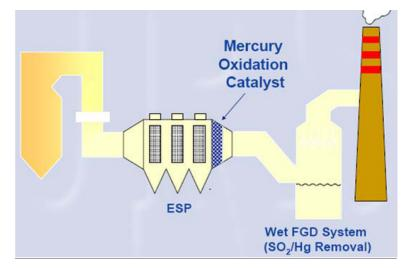
The mercury oxidation catalyst is located between the ESP and the wet FGD where both SO, and mercury are removed.
