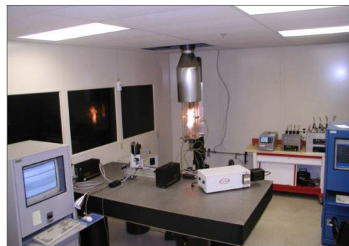
2-D optical sensor positioned for data acquisition from the natural gas test burner
