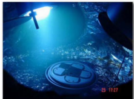
Sputtering deposition in the fabrication of the sensor.
