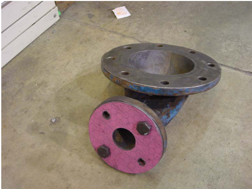
Figure 4.3-20 Original 90° Bend From FD0520
