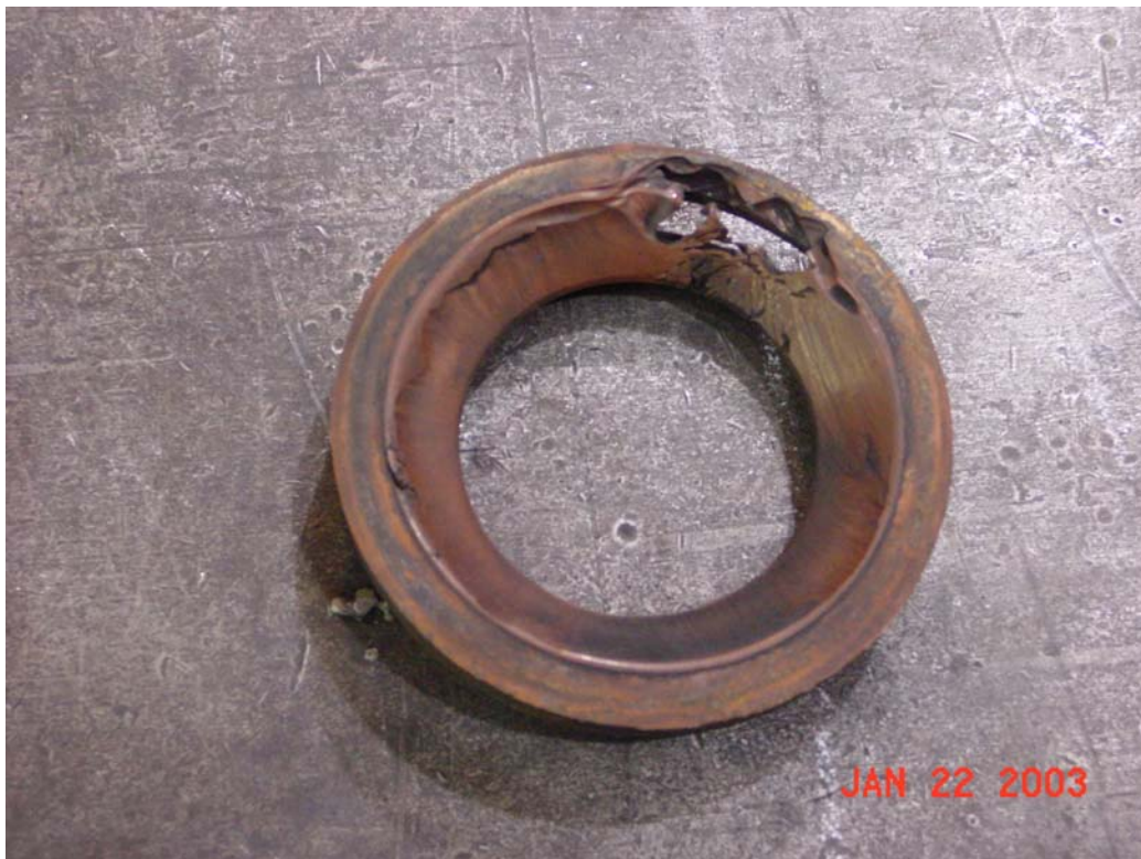
Figure 4.3-22 Outlet Conveying Line Spheri-Valve Seal After TC10
