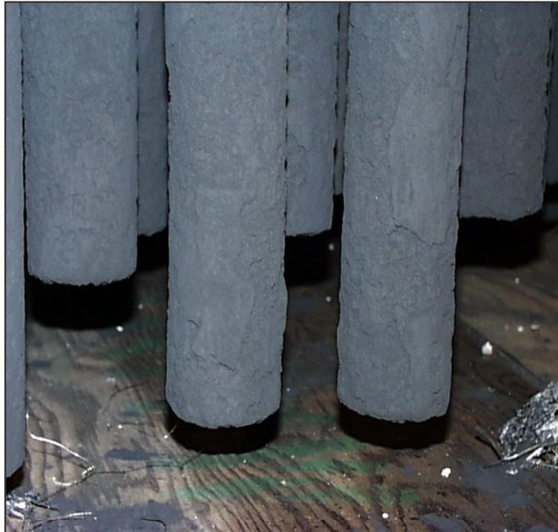
Figure 3.3-18 Bottom Plenum Filter Element Char Cake (GCT1B Through D)
