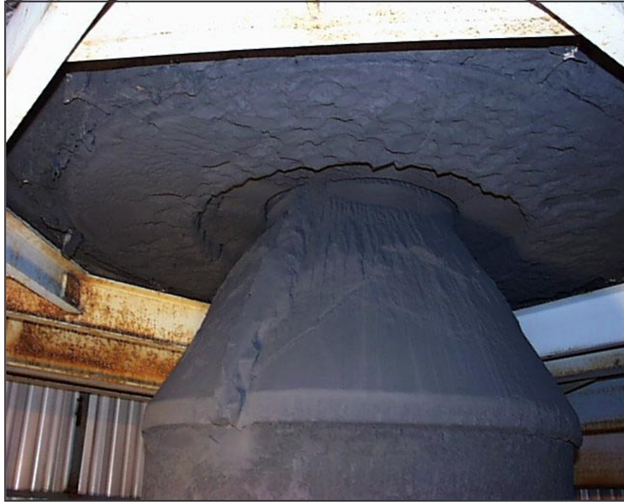
Figure 3.3-19 Char Accumulation on Top Plenum (GCT1B Through D)
