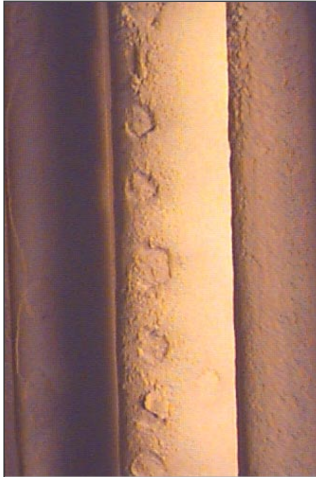
Figure 3.3-7 Membrane Spalling on Honeywell PRD-66 Composite Element (T16)
