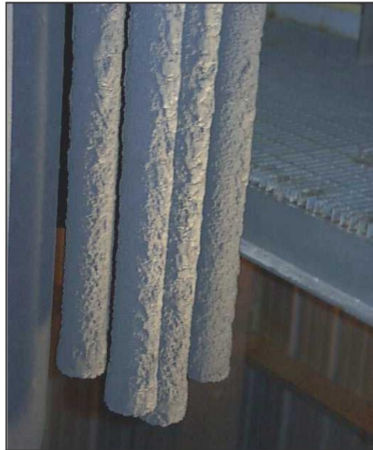
Figure 3.3-17 Top Plenum Filter Element Char Cake (GCT1B Through D)
