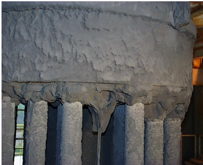
Figure 3.3-20 Char Accumulation on Top Plenum, Top "Ash Shed," and Bottom of Tubesheet (GCT1B Through D)
