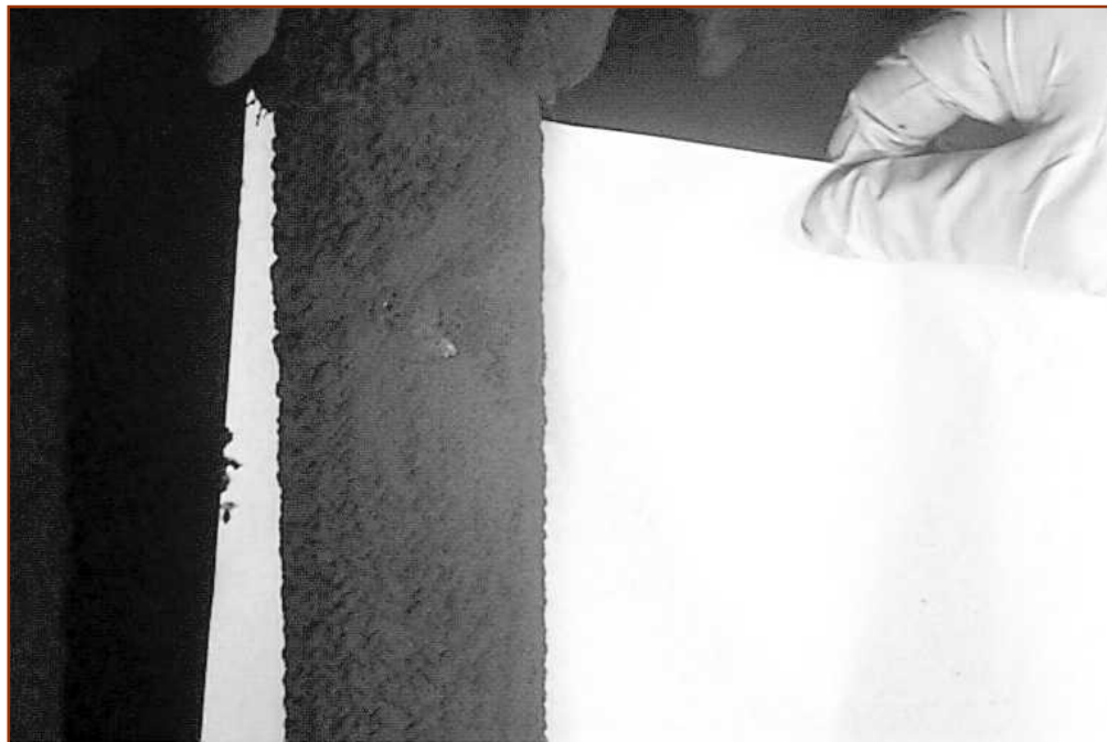
Figure 3.3-6 Potential Leak Paths on 3M Oxide Composite Filter Element (T14)
