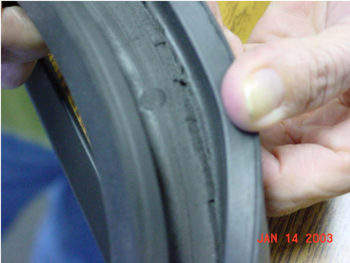
Figure 3.3-16 Cracked Upper Spheri Valve Seal After TC09
