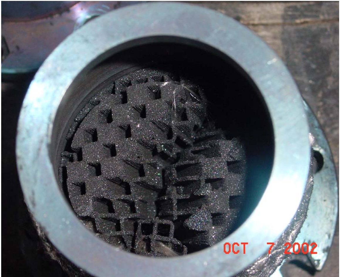
Figure 3.3-10 Specific Surface Failsafe Device After TC09
