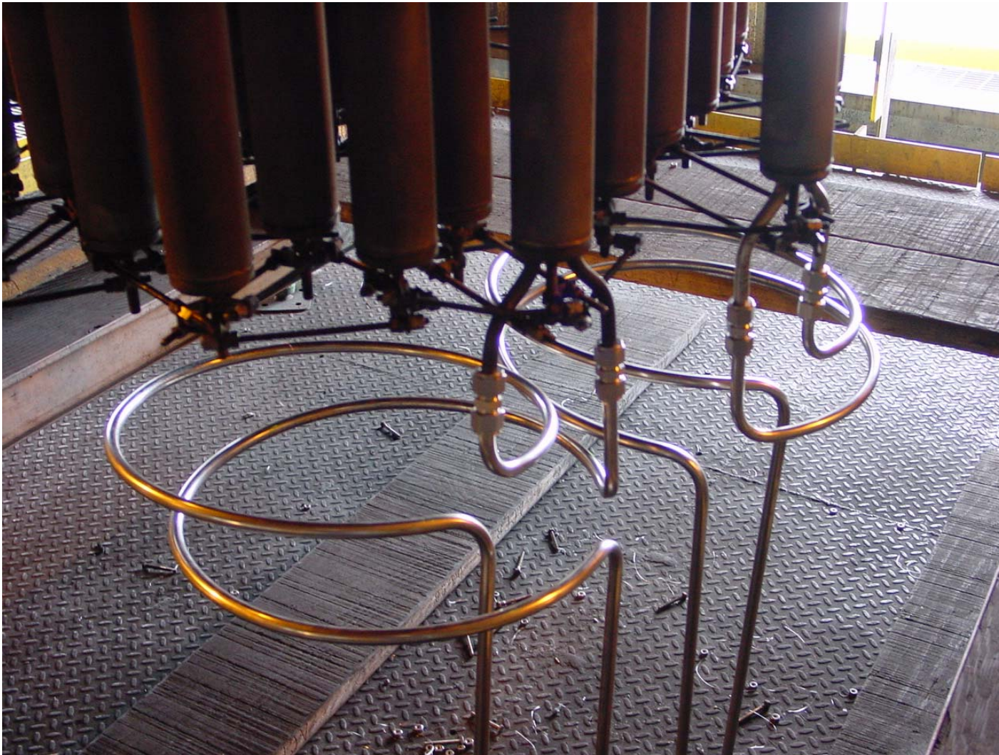
Figure 3.5-3 Modified Filter Elements for Solids Injection Test
