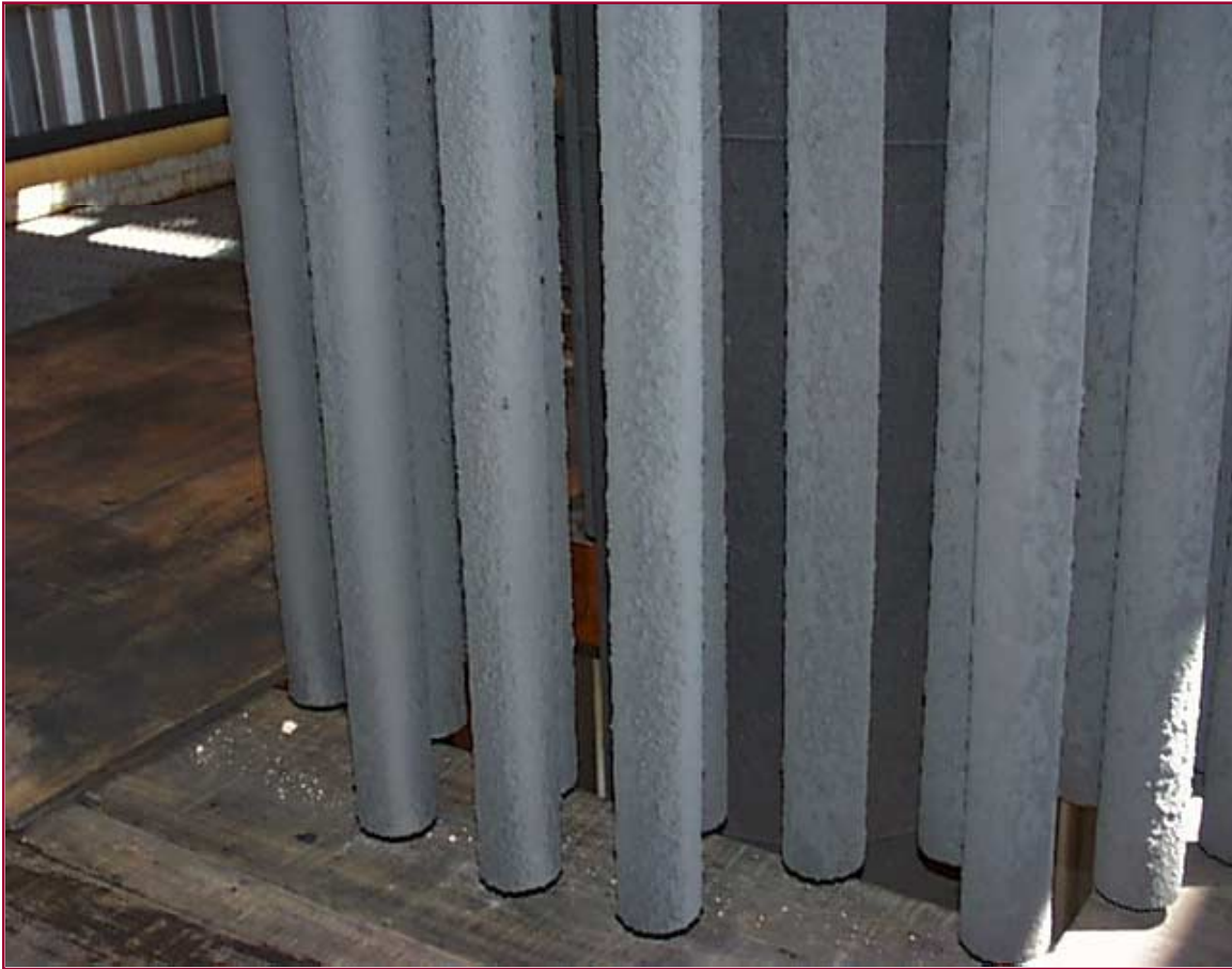
Figure 3.3-6 Char Accumulation on Monolithic SiC Filter Elements
