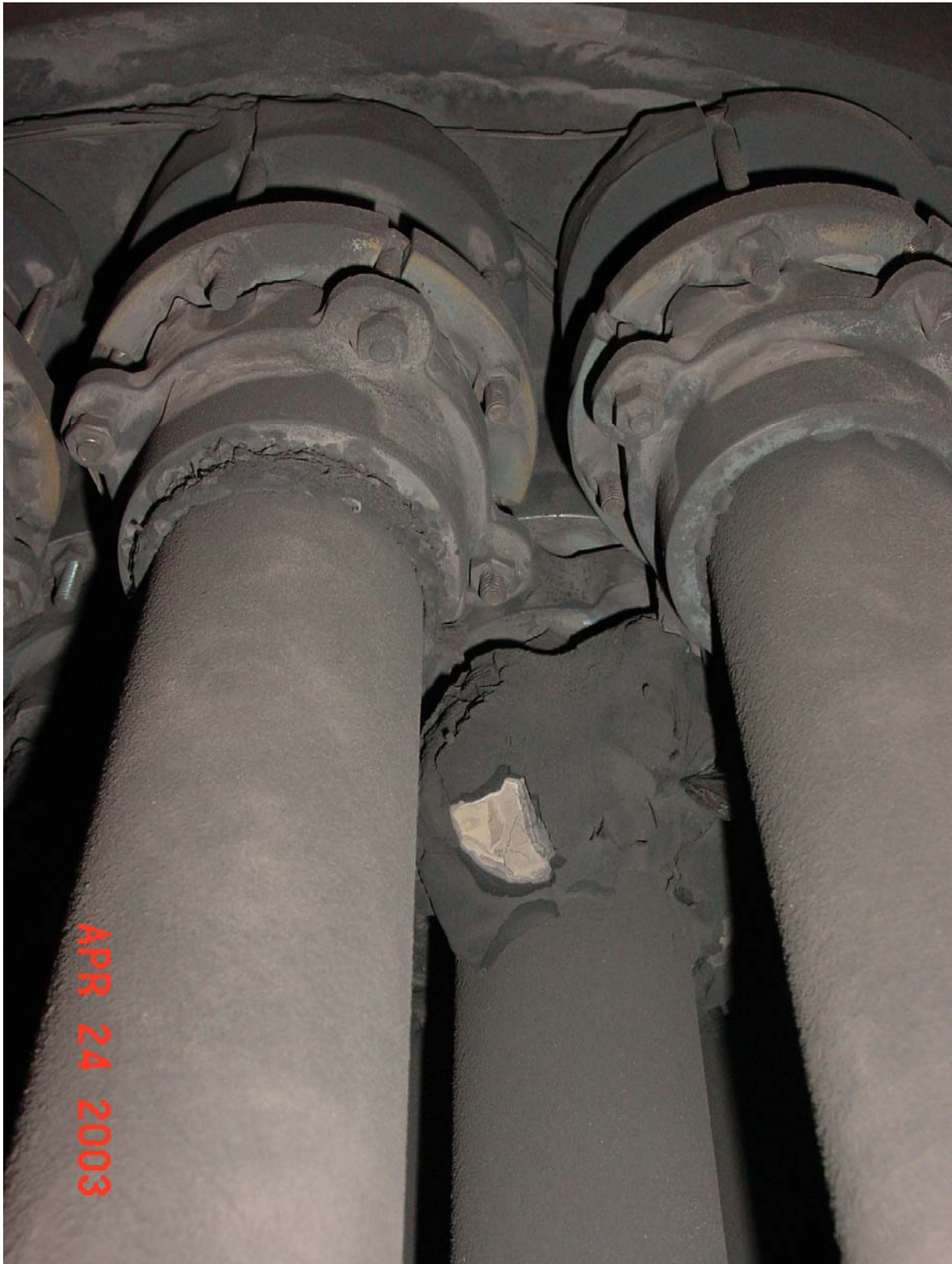
Figure 4.3-3 Solid Deposit on Filter Holder
