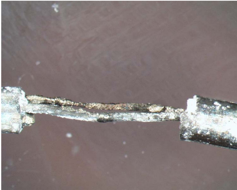
Figure 4.3-10 Side View of Probe Showing Corroded Thermocouple Wire
