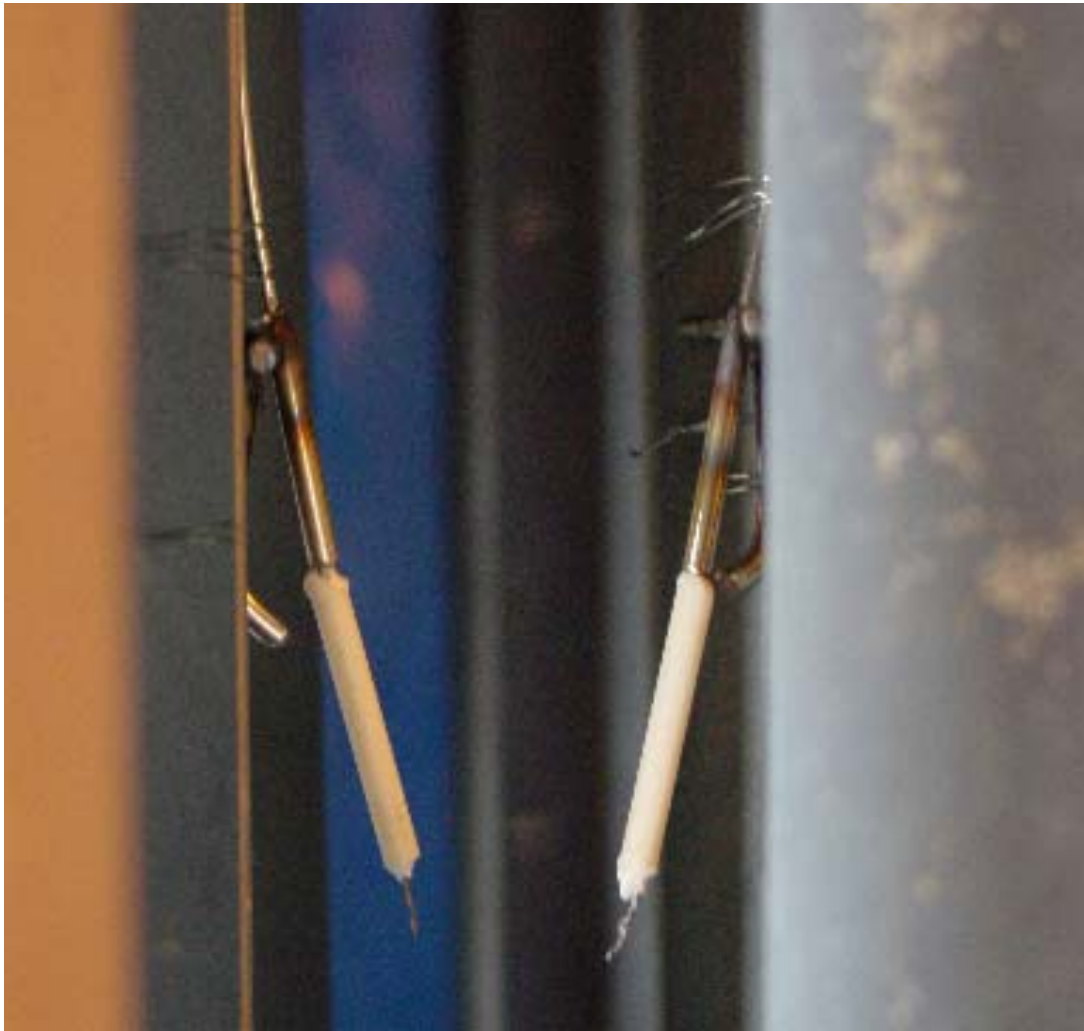
Figure 3.3-26 G-ash Resistance Probes Used During TC07D
