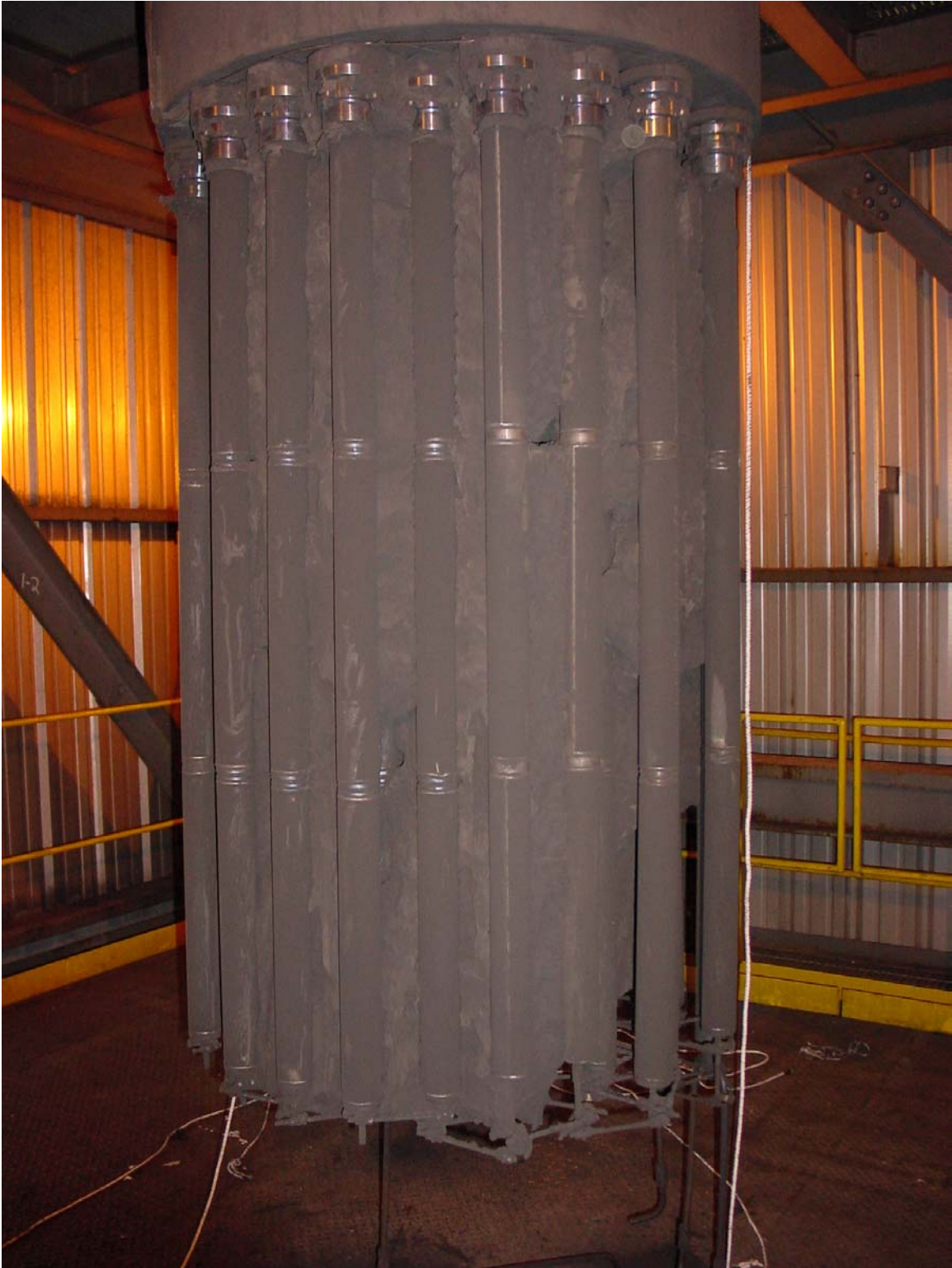
Figure 3-3-4 G-ash Bridging After TC07C
