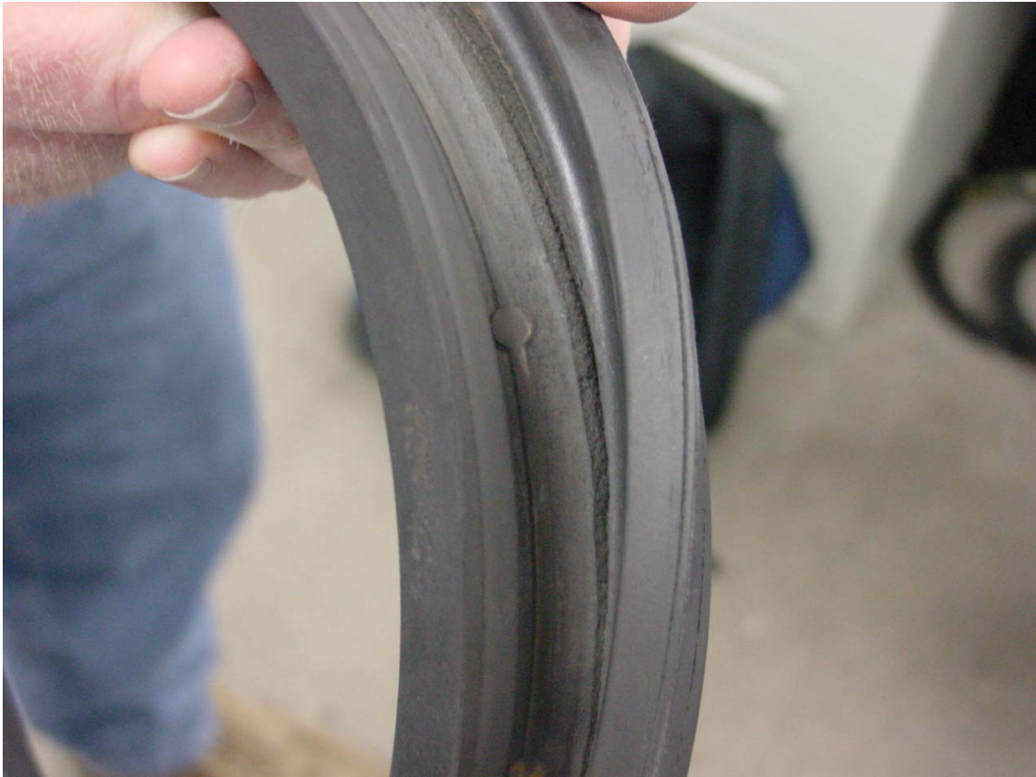
Figure 3.3-31 Cracked Spheri Valve Seal After TC07D
