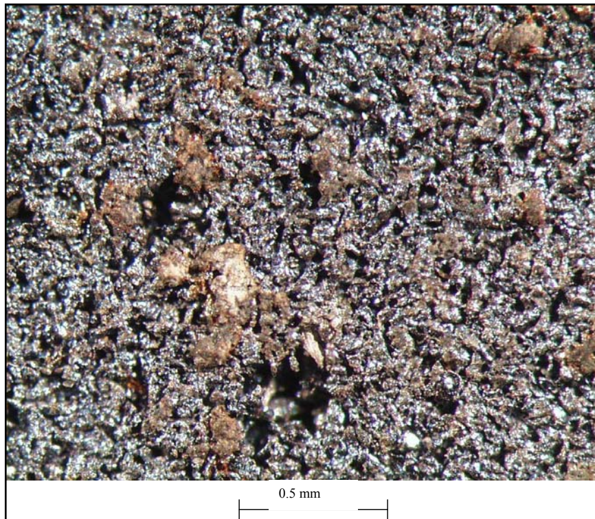
Figure 3.3-11 Pitting on the Outside Surface of Virgin Pall Fe 3 Al Element 22362
