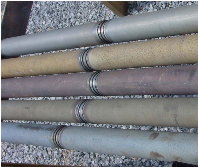
Figure 3.3-7 Typical Pall Fe 3 Al Elements Removed From GCT4 After Cleaning by Pressure Washing
