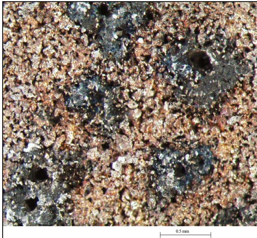
Figure 3.3-6 Pitting on the Outside Surface of Pall Fe 3 Al Element 21080 Removed From Plenum Location B-17 After GCT-4
