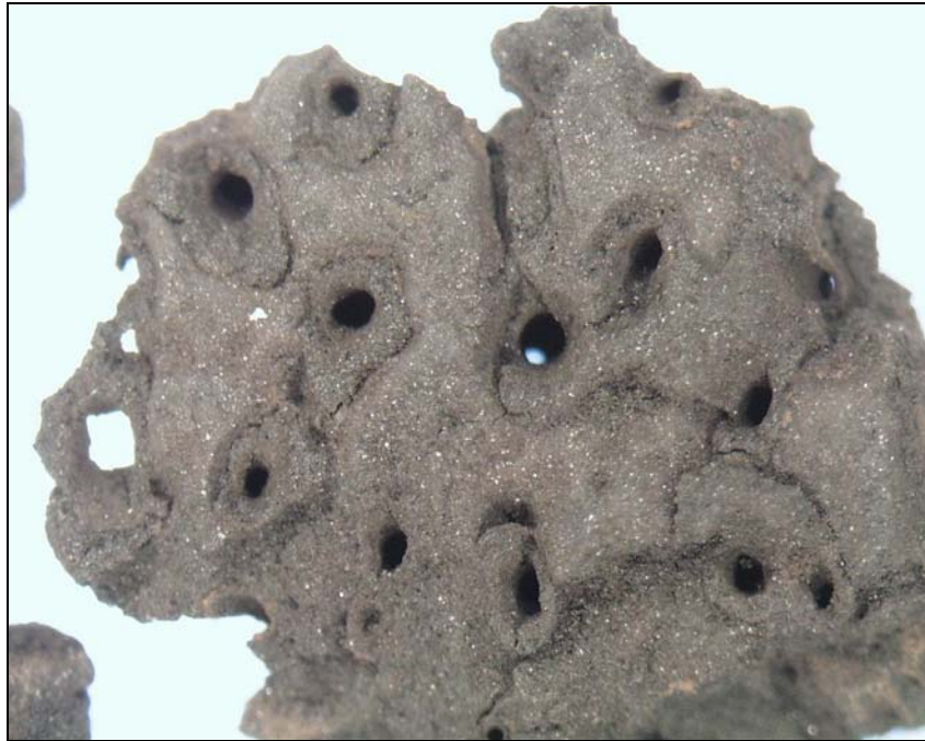
Figure 3.4-1 GCT4 Residual Dustcake at 30x Magnification
