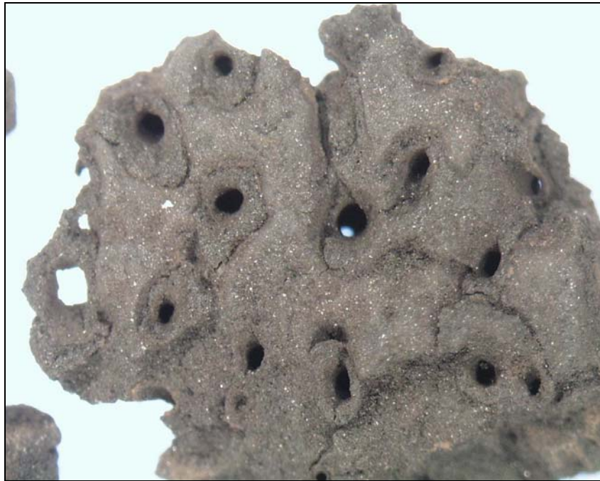
Figure 3.6-1 GCT4 Residual Dustcake at 30x Magnification
