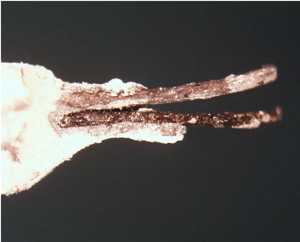
Figure 4.3-9 Corroded Resistance Probe After TC12
