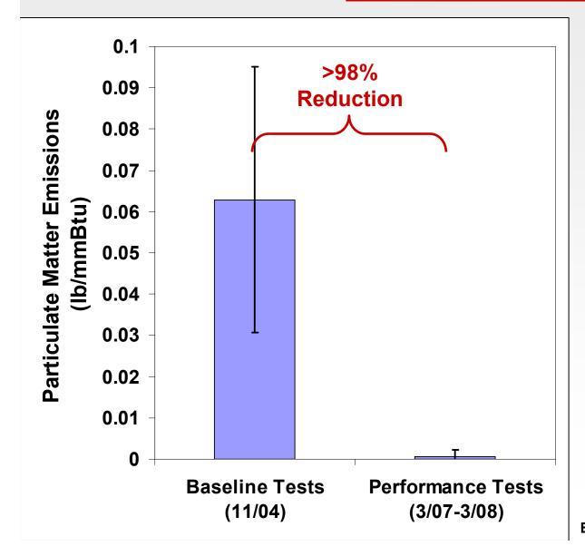
New baghouse significantly reduces particulate matter emissions relative to old ESP, in spite of increased particle loading from Turbosorp® scrubber
