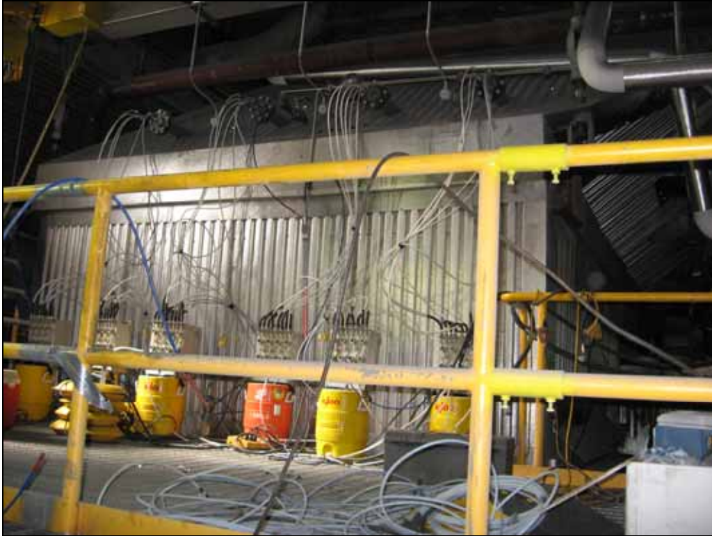
Figure 4. Photograph of sampling at the SCR inlet and outlet grids. Grid-point NO x sampling was performed by Clean Air Engineering.
