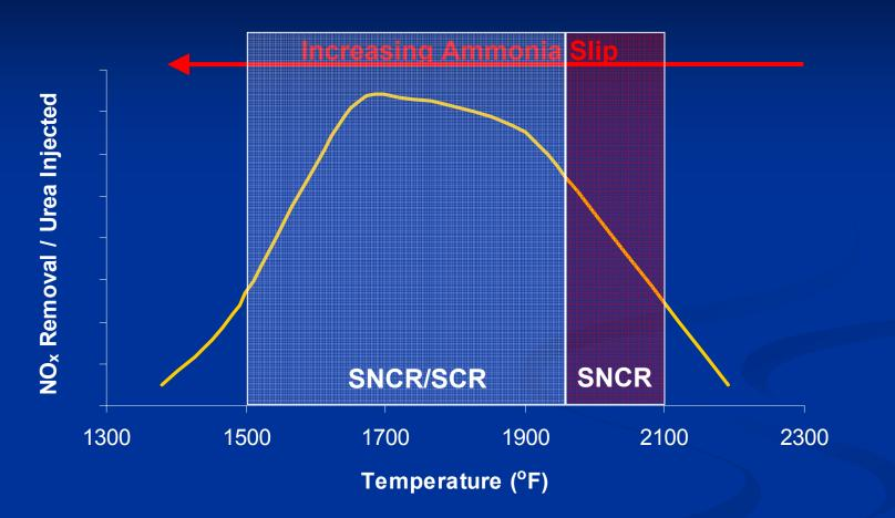
Hybrid SNCR operates at lower temperature than stand-alone SNCR
