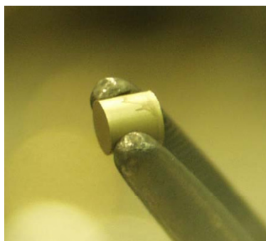
Inert Matrix Fuel (IMF): (\text{Zr}_{0.58}\text{Pu}_{0.21}\text{Am}_{0.21})\text{N}
