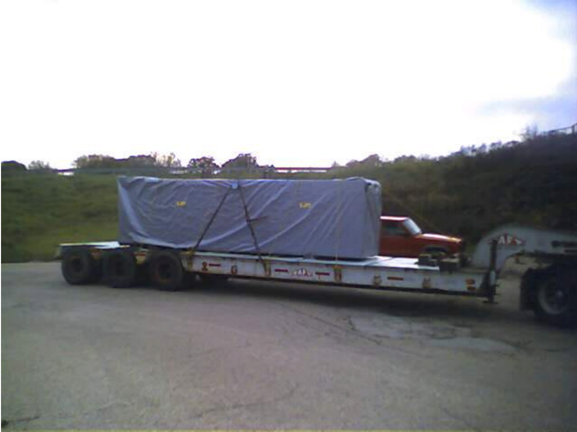
MiniBooNE Horn Contained Inside Wrapped Steel Coffins for Transport to Storage Building
