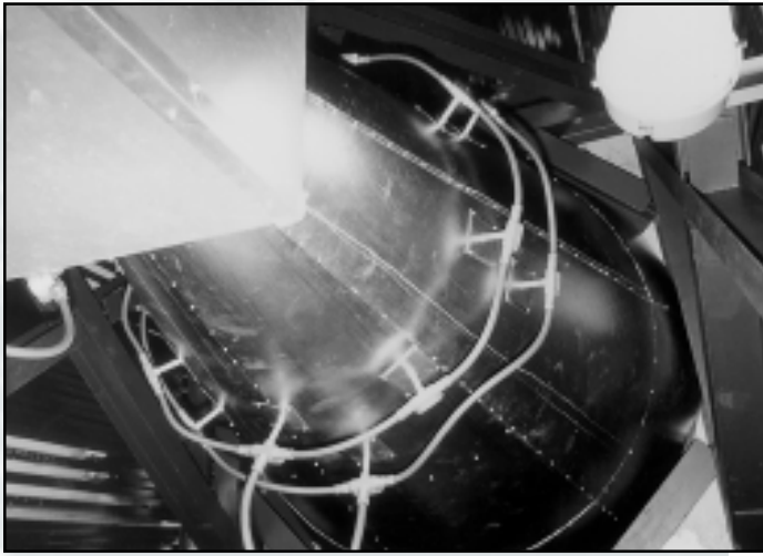
Bottom of cyclone separator where it attaches to collection box; captured solids are either recycled to GSA or drawn off as waste
