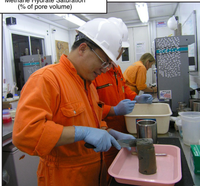
Dr. Nengyou Wu cleans a sediment sample before squeezing it for sedimentary porewater. Freshening noted in porewater samples is one method used to calculate gas hydrate concentration (above).
