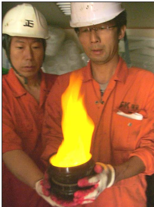
Methane from recovered gas hydrate sample is set alight during coring operation.
