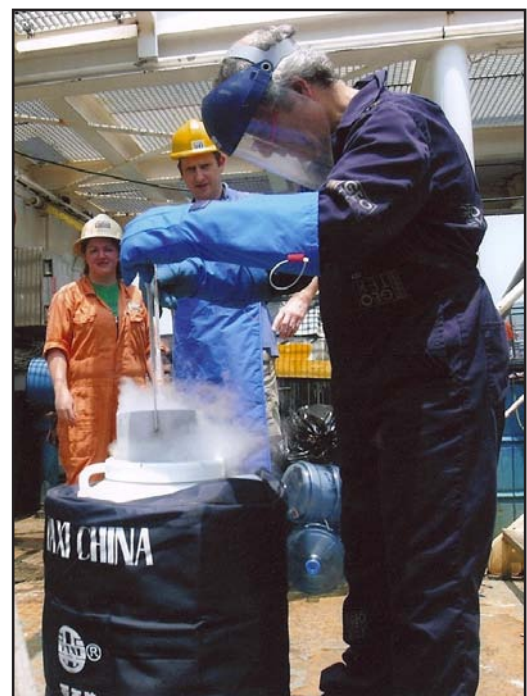
Gas-hydrate-bearing sediment samples being transferred into liquid nitrogen for delivery to GMGS.
