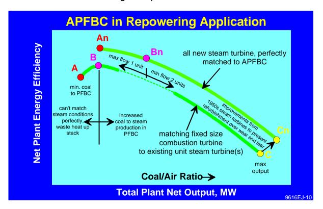
It is unlikely that the steam turbine will match exactly the thermal integration needs operation at the "A" operating point, where the combustion turbine power output is large relative to the steam turbine power. Exhibit 8 shows the likely circumstances for a repowering, compared to the same combustion turbine that has been perfectly matched to an all new steam turbine system "An."
