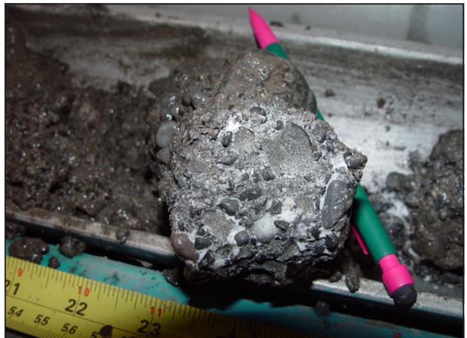
Gas hydrate-bearing sediment core from the Mallik site, Northwest Territories, Canada.
