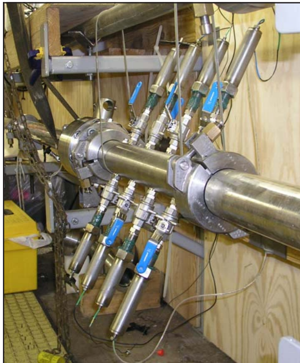
This device, constructed by Georgia Tech in association with the GOM JIP, enabled the first physical property measurements to be made on a deep-sea hydrate core consistently maintained at in-situ pressures.
