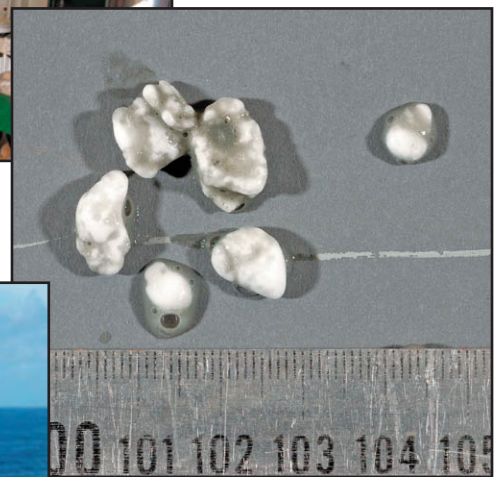
Hydrate samples fizzing and bubbling as they decompose at ambient conditions.
