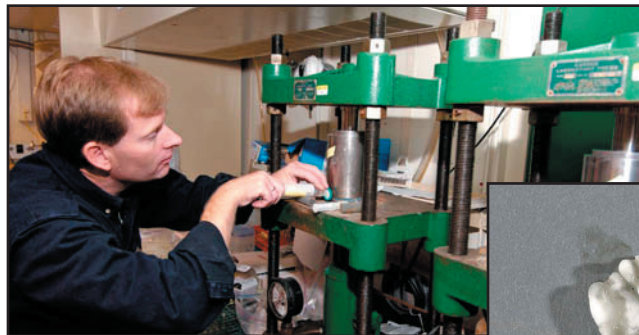
Geochemist squeezes a core sample to extract the interstitial water for chemical analysis.
