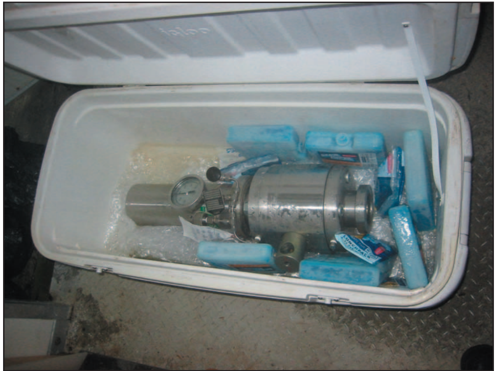
• Pressure vessel containing a natural sediment sample recovered during the 2005 Gulf of Mexico Joint Industry Project (JIP) drilling cruise that has not been depressurized.
