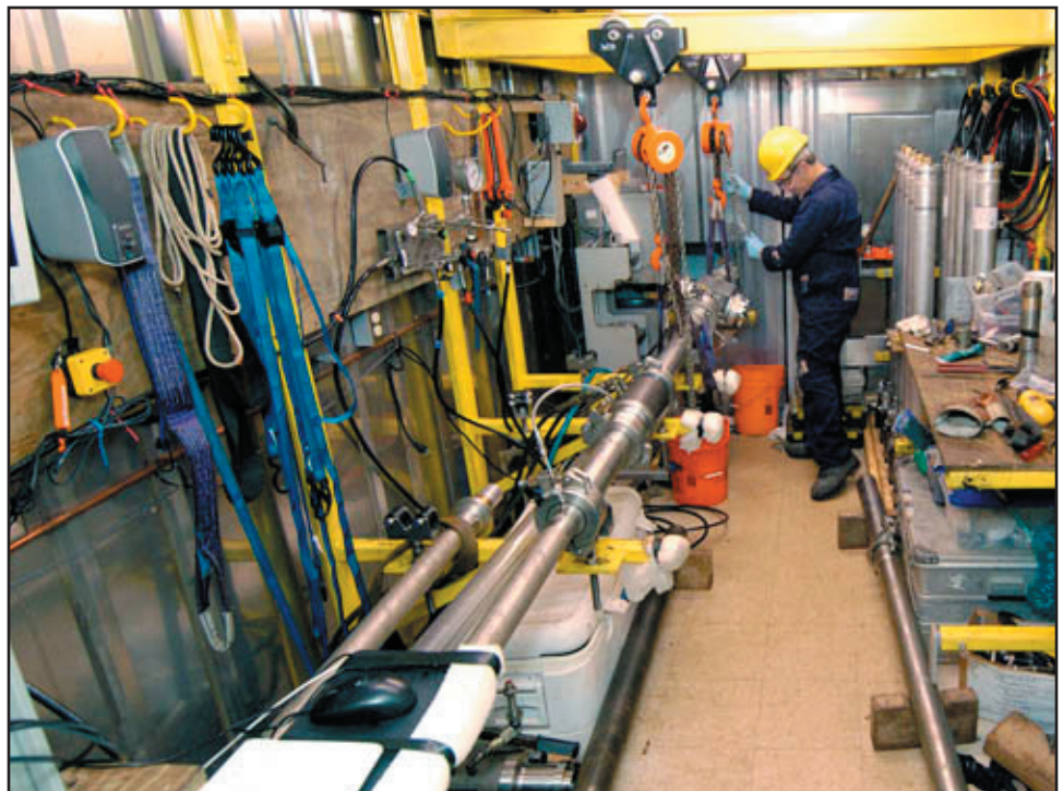
Pressure Core Specialist manipulates a pressure core recovered during the IODP Expedition 311.
