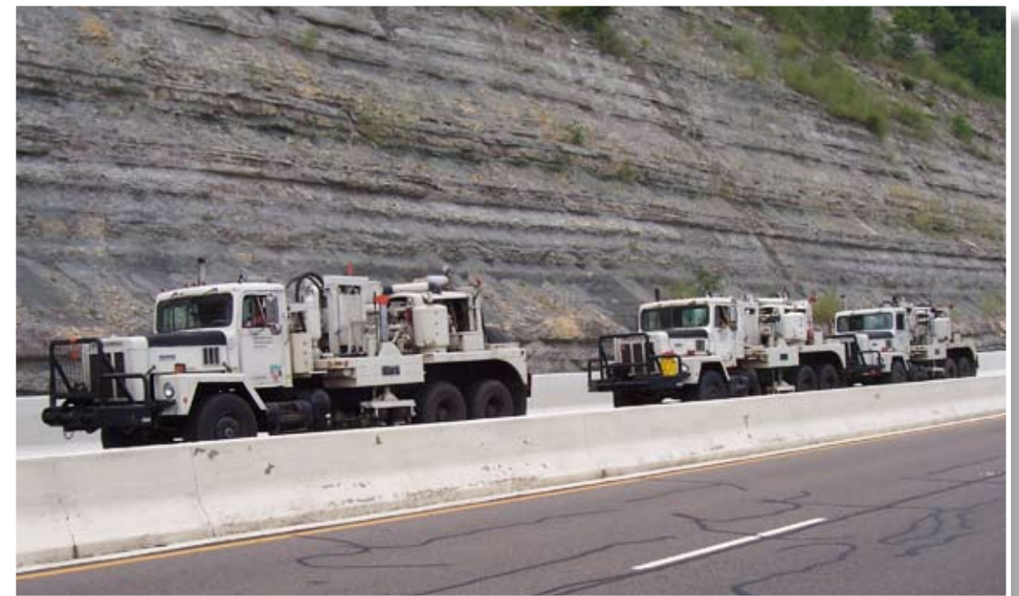
Seismic survey trucks move along a rock outcrop at the Appalachian basin R.E. site.
