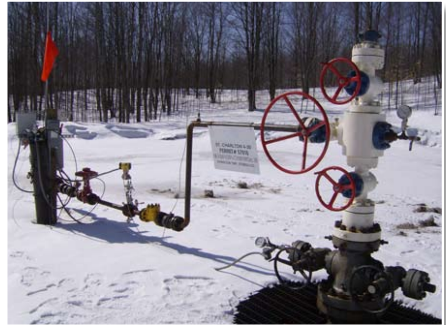
The MRCSP Michigan basin field test was concluded in March 2008 after successful injection of 10,241 metric tons CO 2 into a deep saline rock formation called the Bass Islands Dolomite at a depth of 3,400–3,500 ft.
