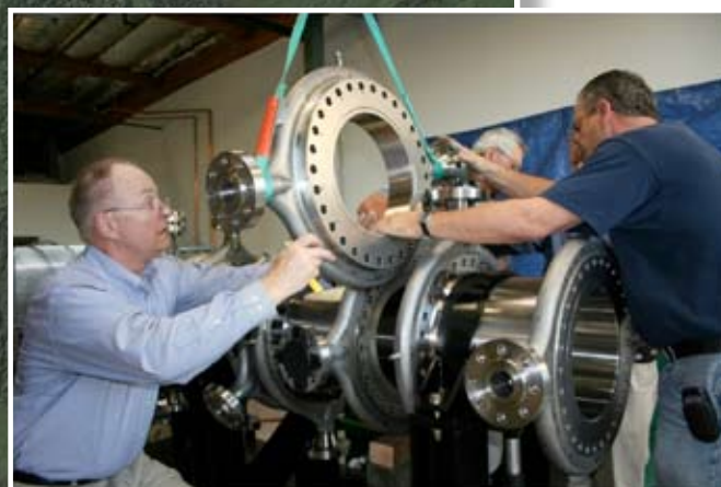
Assembling the diluent injector in Clean Energy Systems’ gas generator (combustor and gas cooler).
