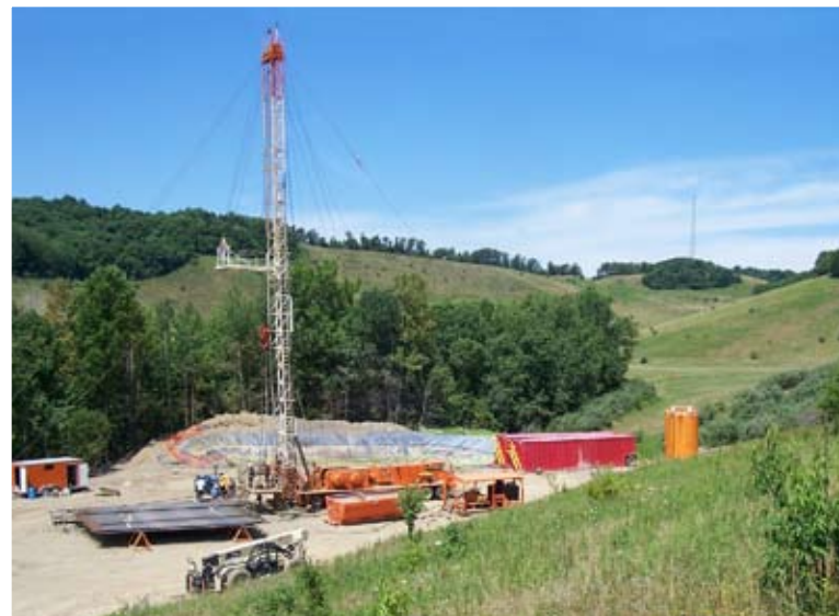
Drilling operations at the Ohio CO 2 sequestration test well in Tuscarawas County, Ohio.
