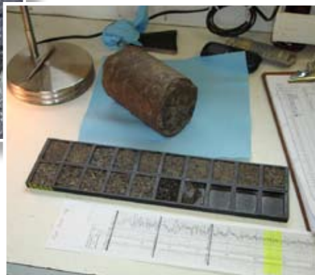
Drill core and drill chip logging from site characterization at the Mississippi Power test site. Courtesy of Southern Company and ARI.
