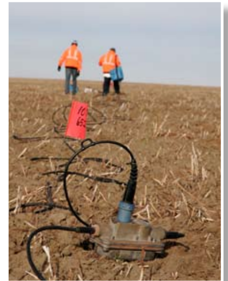
Placement of survey equipment at a proposed basalt field site.
