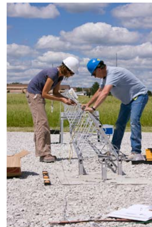
Setting up the Eddy Covariance tower at the Illinois Basin – Decatur site.
