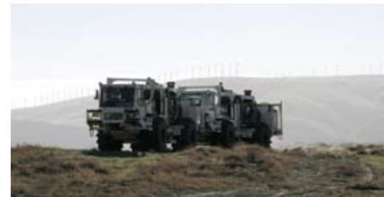
Thumper trucks deliver seismic energy to the subsurface to detect underground faults.
