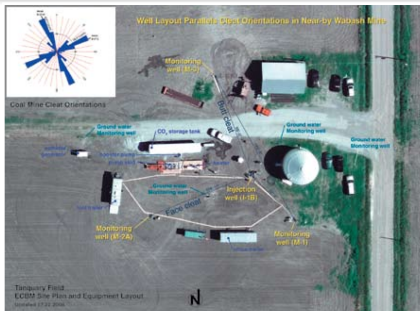
Layout of coal test site. Inset shows coal cleat orientation at a nearby mine.
