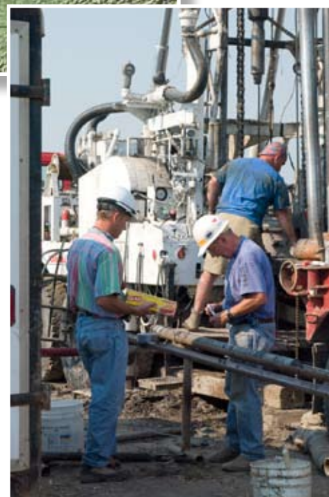
Collecting core at coal test site.
