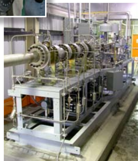
Assembling the diluent injector in Clean Energy Systems’ gas generator (combustor and gas cooler).
