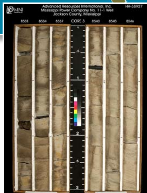
Drill core collected from Tuscaloosa Formation beneath Plant Daniel. (Courtesy of Southern Company and ARI.)
