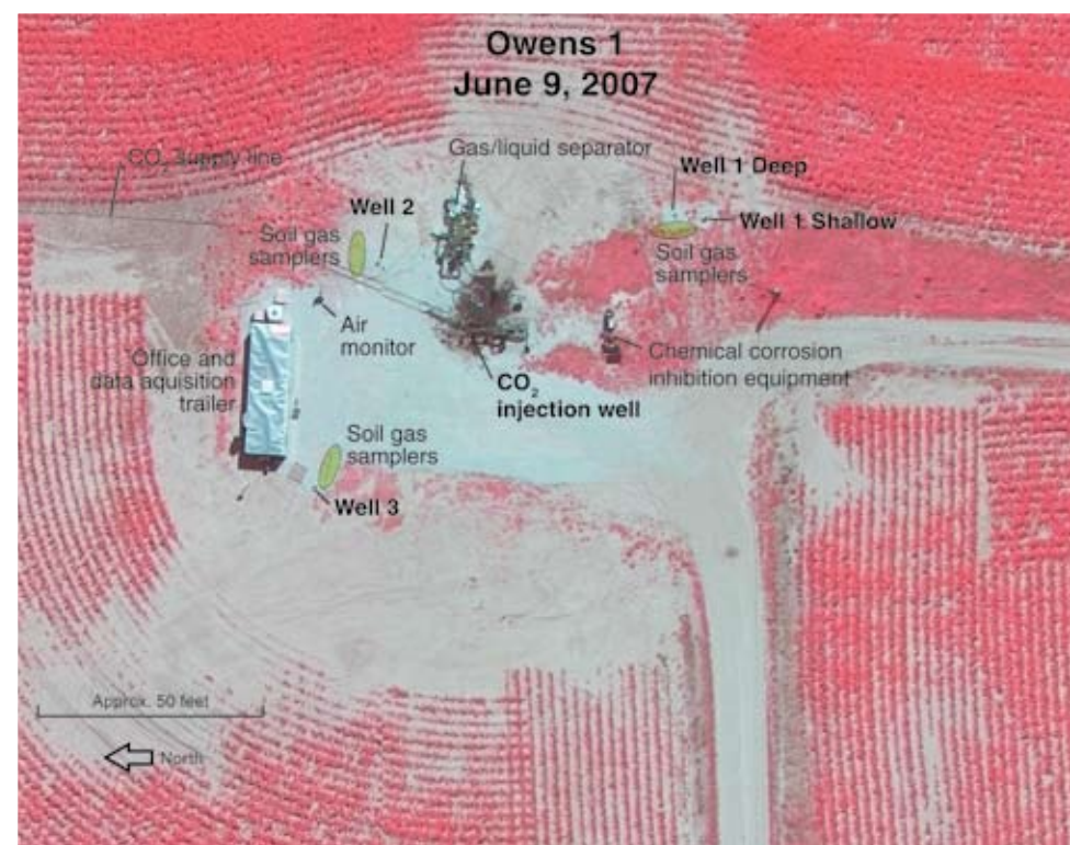
Layout of EOR I site in the Loudon oilfield, Fayette County, Illinois.
