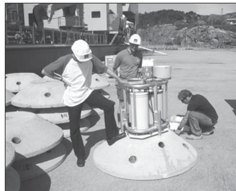
Gravimeter array shown with sea floor concrete monuments prior to emplacement
