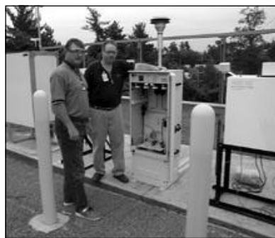
NETL scientists standing at the Andersen speciation sampler used to collect fine particulate matter
