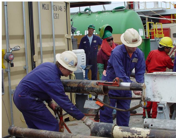
Moving the Coring Assembly to the Core Processing Container
